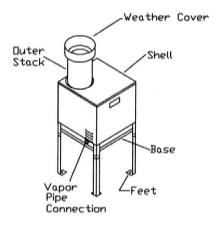
Balance Phase II EVR System for Protected Aboveground Storage Tanks Exhibit 8 - VR-501-E
