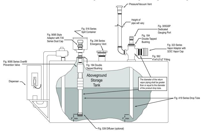
Tank gauging may be done by way of a mechanical gauge (Fig 818 or 918 Series) or an electronic gauge (Fig 305 Series)"
