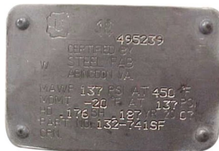
Clean Air Separator Data Plate (not pictured on far side of base)
