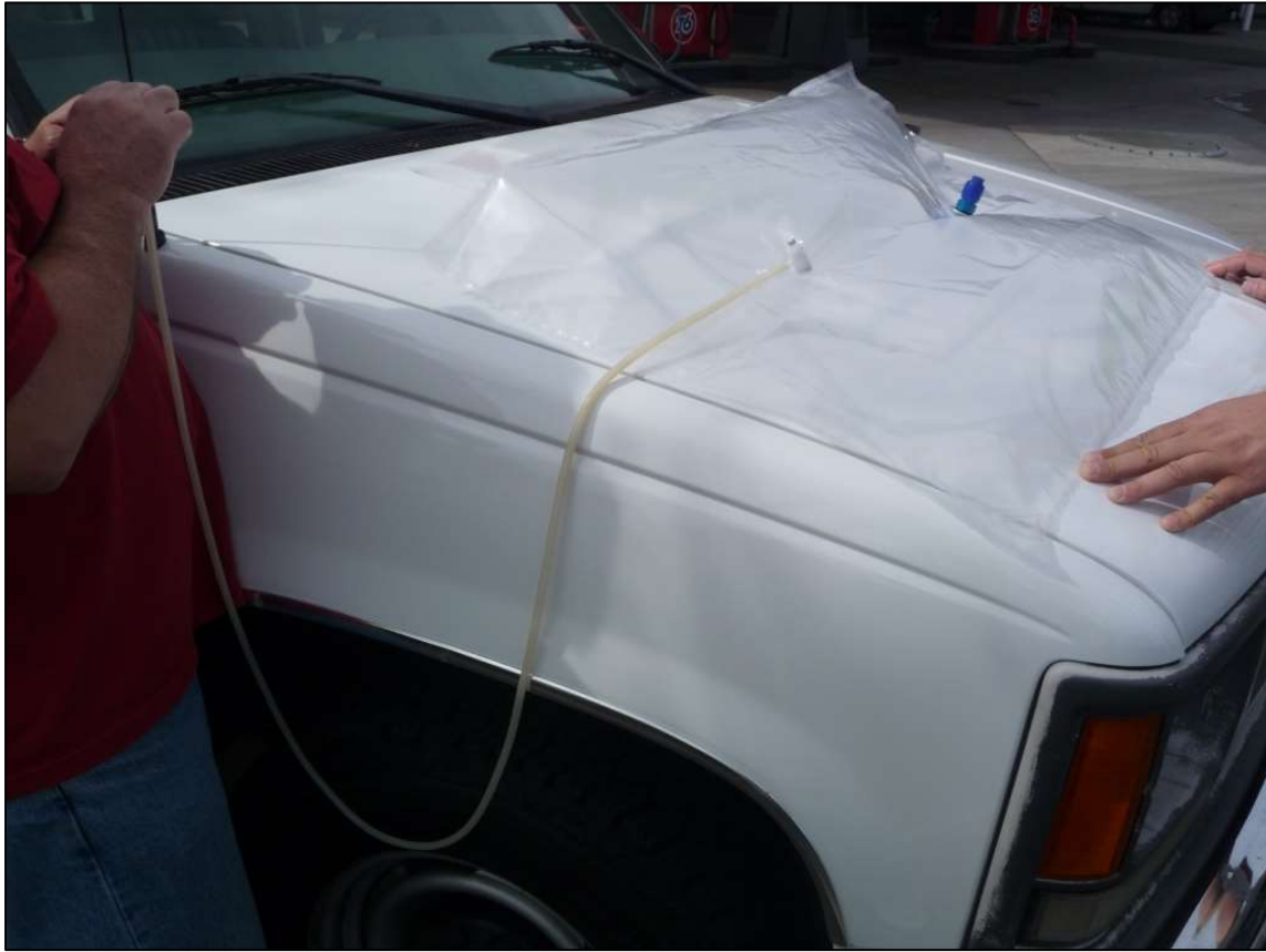
FIGURE 15- 2 Tedlar Bag Connected to Nitrogen
