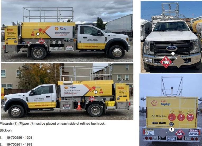
Placards (1) (Figure 1) must be placed on each side of refined fuel truck.
