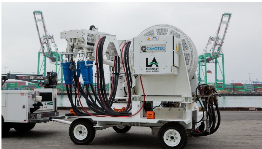
Figure 3. Proposed cable management system.
