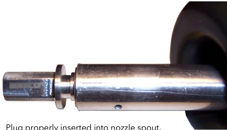
Plug properly inserted into nozzle spout.
