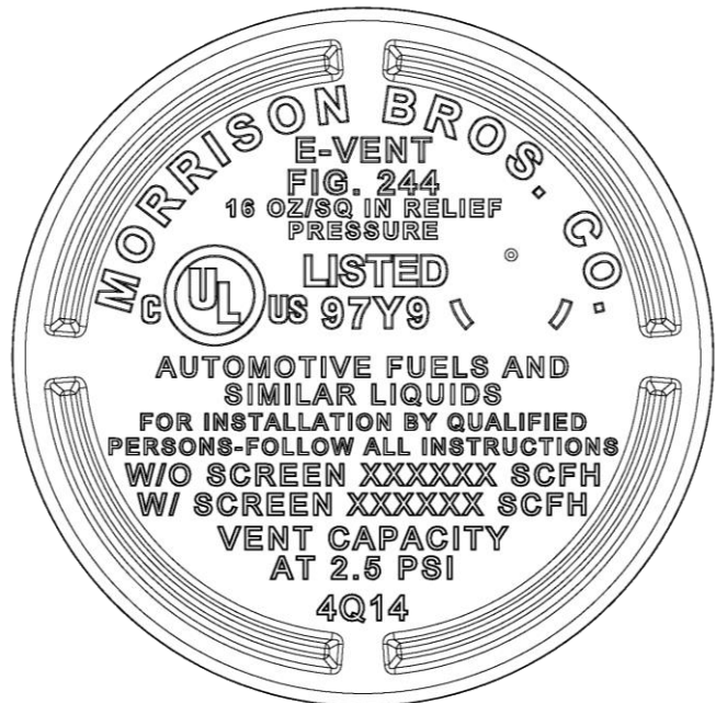
Vent Sample With Relief Opening Pressure Greater Than or Equal to 0.5 Psi
