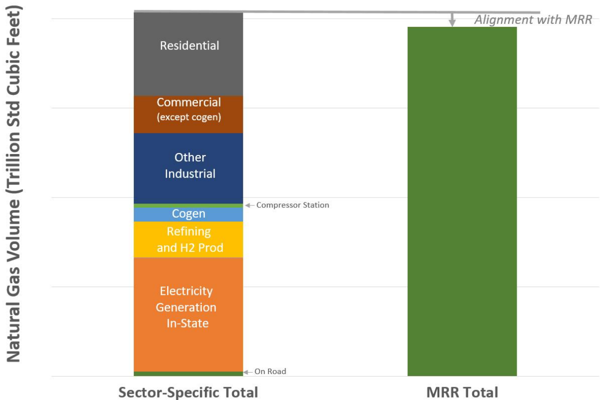
Figure 3: An Illustration of Natural Gas Combustion Categories Within the Scope of MRR Section 95122 Reporting and Alignment with MRR Total Volume
