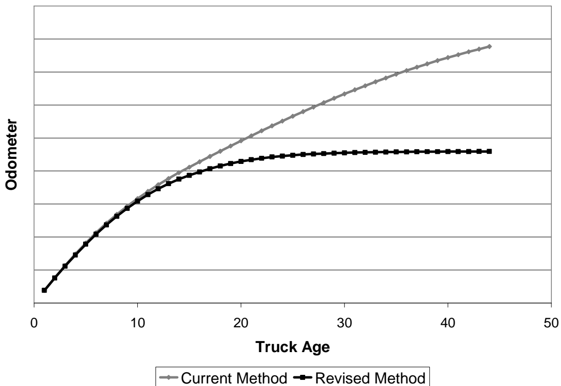
Figure 5. Schematic Representation of Difference between Current and Revised Method for Estimating Vehicle Odometer
