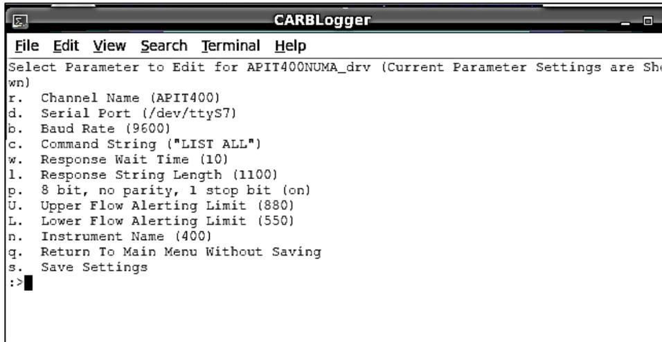
Figure 3.6: Common Editable Parameters from an Instrument Driver
