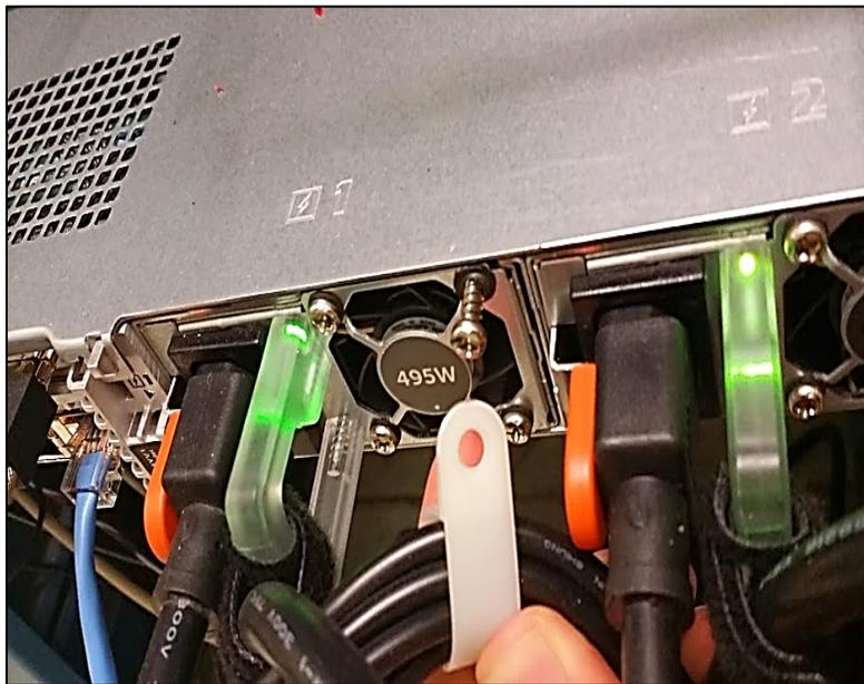
Figure 2.2: Securing Cables to CL Chassis.
