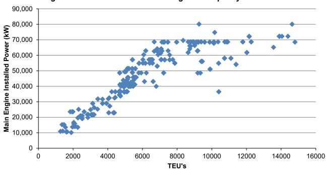
Figure 6: Container Vessel Main Engine to Capacity in 2014
