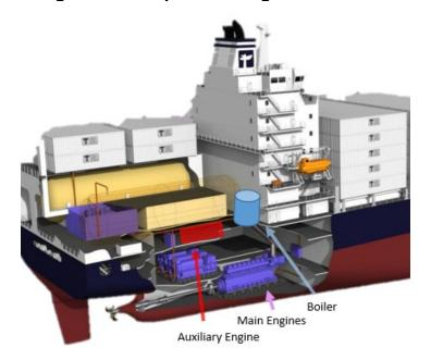
Figure 1: Example OGV Engine Illustration
