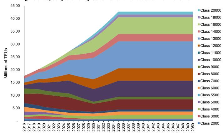
Figure 5: Capacity Growth by Container Size Forecast for POLA and POLB
