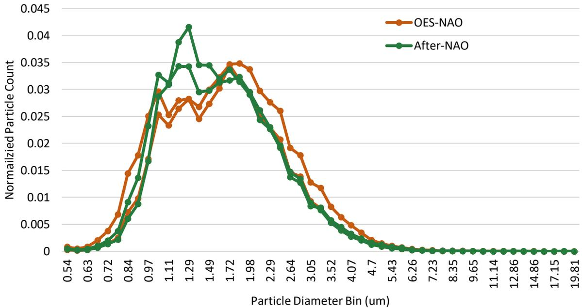
**Figure 67. Size distribution of Prius front brake PM as measured by APS**
