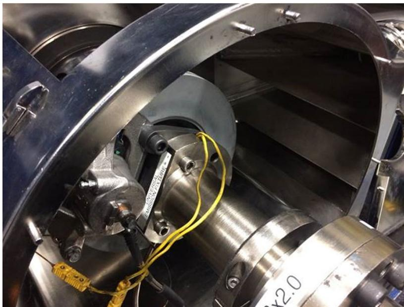
**Figure 19. A brake rotor installed in the LINK test enclosure.**
