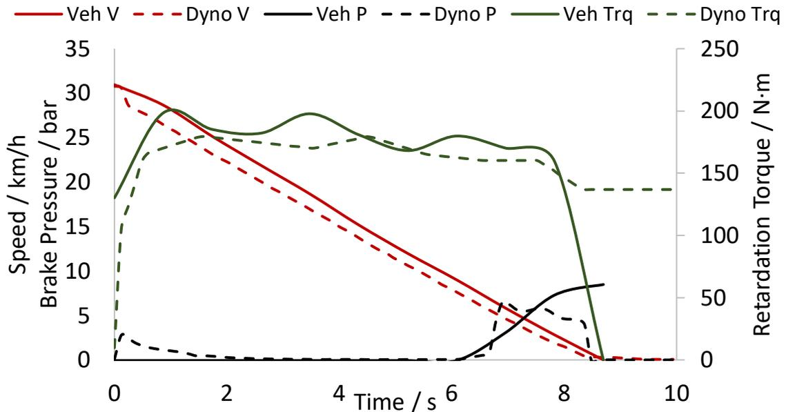
**Figure 23. Dynamometer-to-track comparison of velocity, brake pressure, and wheel torque for example regenerative braking events**
