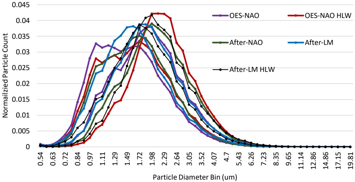
**Figure 66. Size distribution of F-150 rear brake PM as measured by APS**
