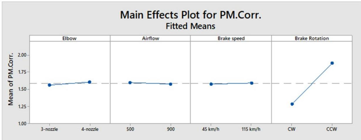
**Figure 35. Graphical plot of the PM response to the parameters of the number of sampling nozzles, airflow rate, brake rotational speed, and brake rotational direction during the Arizona dust evaluation**
