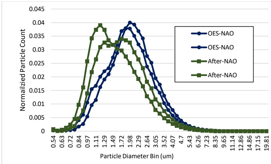
**Figure ES-4. Particle size distribution for the Civic Front axle tests, 0.5-18  $\mu\text{m}$ .**
