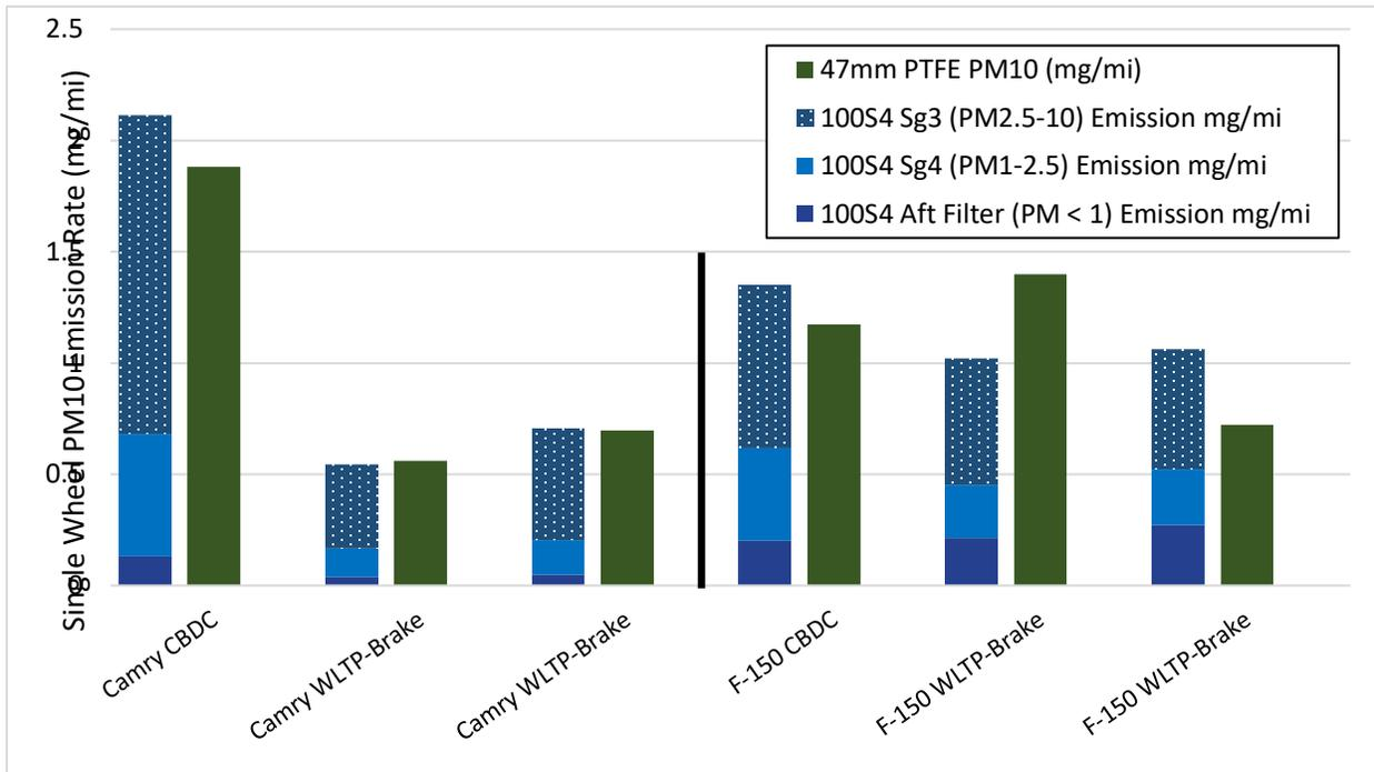
**Figure 83. Comparison between the CBDC average results to replicate tests of the WLTP-Brake for the OES-NAO materials for the Camry and F-150 front axles**
