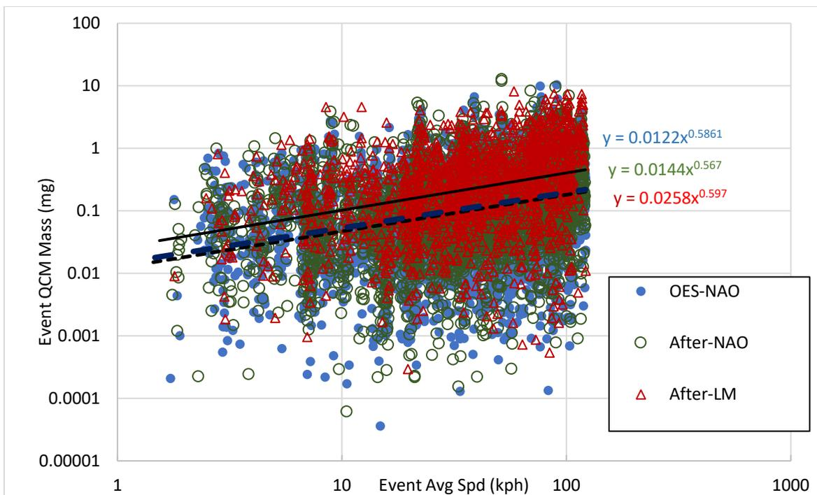
**Figure 75. Trends in QCM brake event PM mass against braking event average speed, categorized by friction material**
