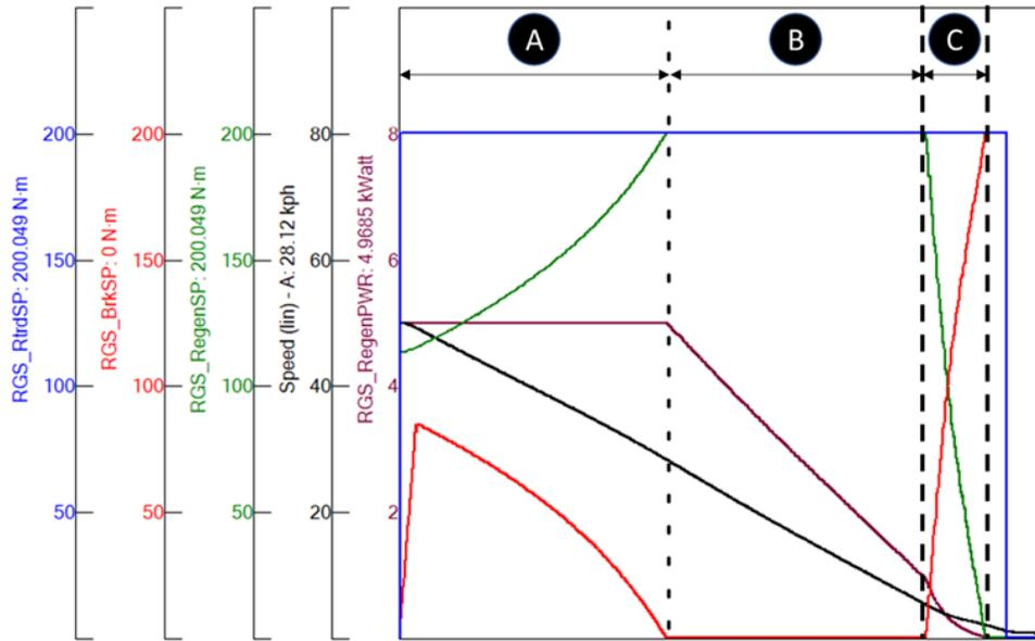
**Figure 22. Plot of retarding torque (blue), friction brake torque (red), regenerative torque (green), wheel speed (black), and regenerative power (purple) during a regenerative-equipped braking event.**
