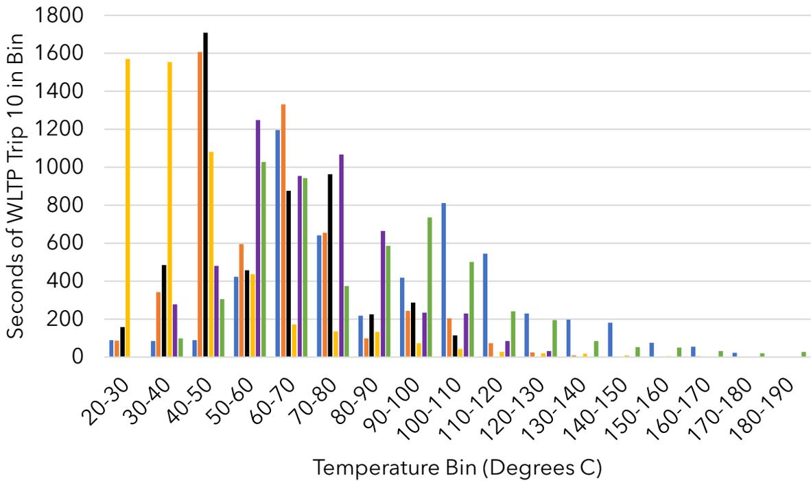
**Figure 5. Histograms of temperatures of front rotors (top) and rear rotors/drums (bottom) over the WLTP-Brake cycle operated on the test track.**
