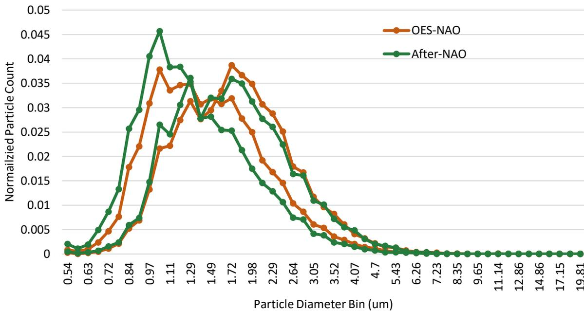
**Figure 68. Size distribution of Prius rear brake PM as measured by APS**
