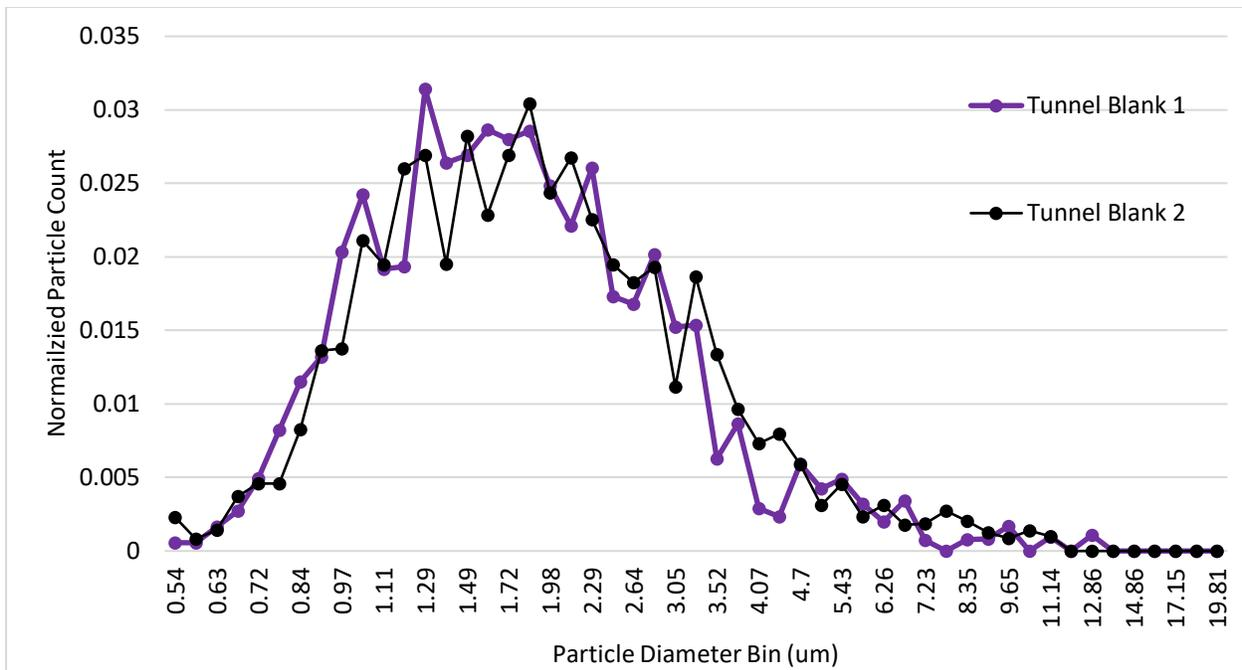
**Figure 73. Size distribution of Tunnel Blanks as measured by APS**
