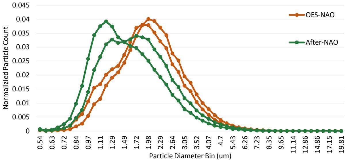
**Figure 63. Size distribution of Civic front brake PM as measured by APS**
