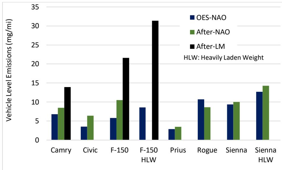
**Figure ES-1. Vehicle level braking emissions by model and friction material**
