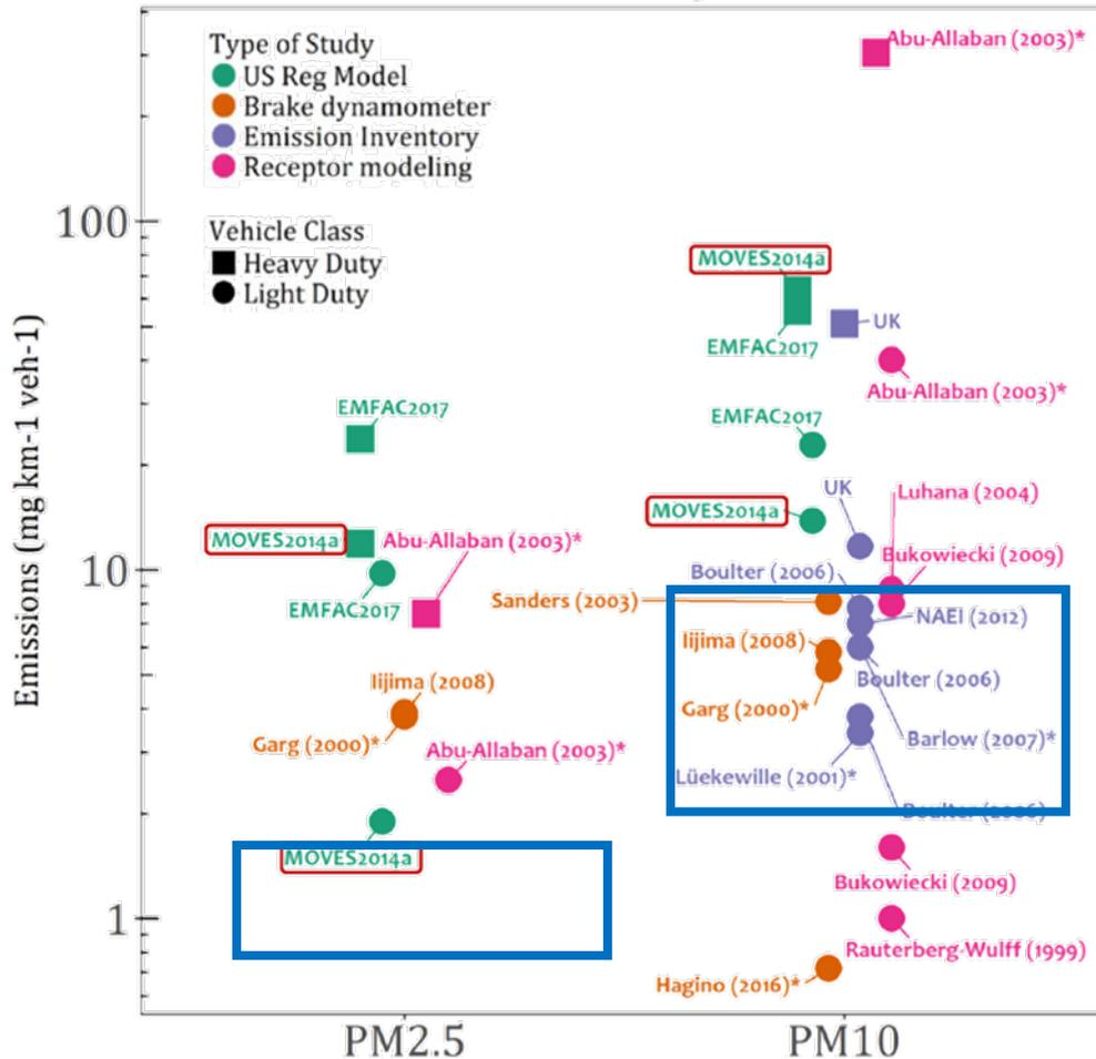
**Figure 96. Various literature values for brake emissions, with the ranges from this study overlaid for comparison**
