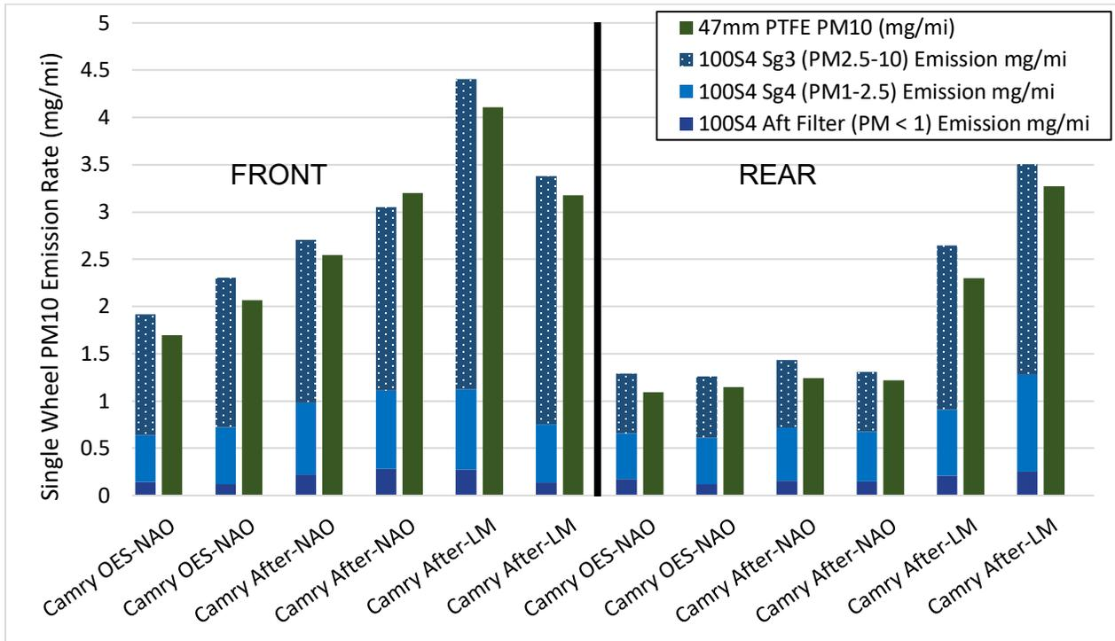
**Figure 40. Single-wheel PM Mass Emission Rates for Camry as measured by 100S4 (Blue) and 47mm Teflon filter (Green)**
