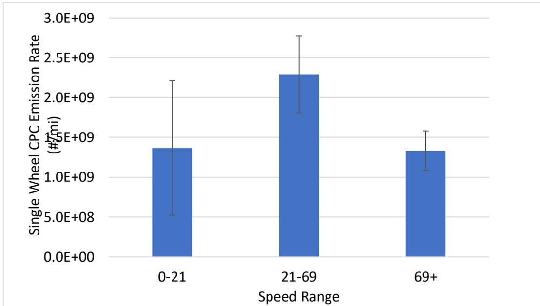
**Figure 60. Overall average single-wheel particle number emission rate across the three speed ranges**
