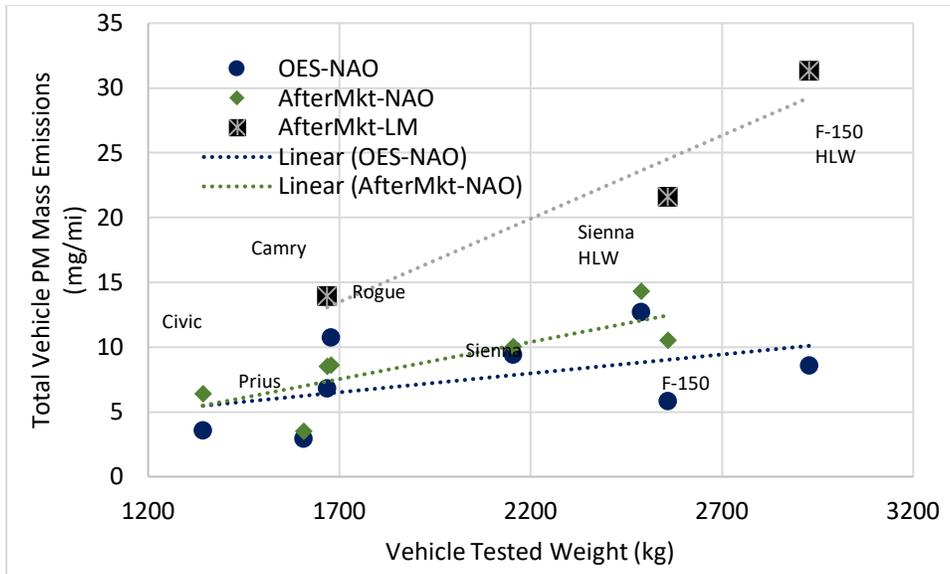
**Figure ES-2. Vehicle level braking emissions vs vehicle test weight by pad material**
