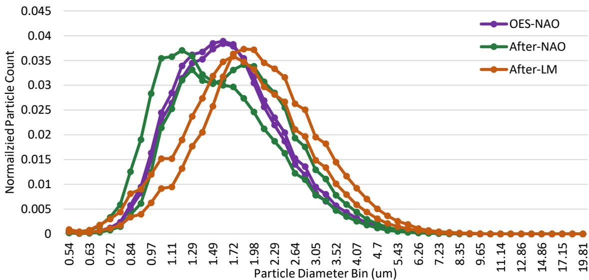
**Figure 62. Size distribution of Camry rear brake PM as measured by APS**
