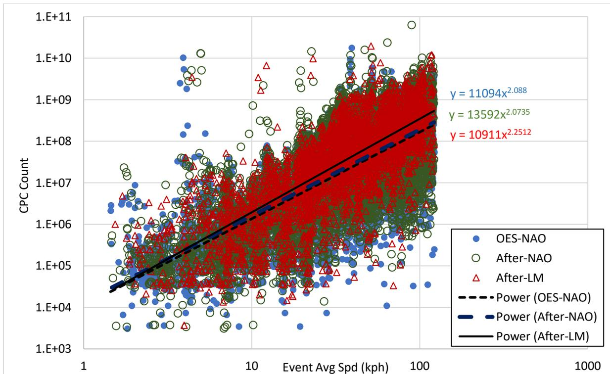
**Figure 74. Trends in CPC count against braking event average speed, categorized by friction material**
