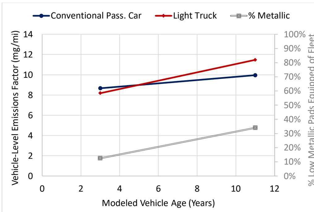
**Figure 98. Emission factor deterioration with vehicle age for conventional passenger cars and light trucks. Also presented is the estimated percentage of in-use vehicles at a given age equipped with LM pads (same for both vehicle types).**
