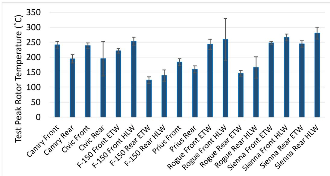
**Figure 38. The peak rotor temperature during the CBDC, averaged across tests by model, axle and test weight. Error bars show the 95% confidence interval of the mean of tests**
