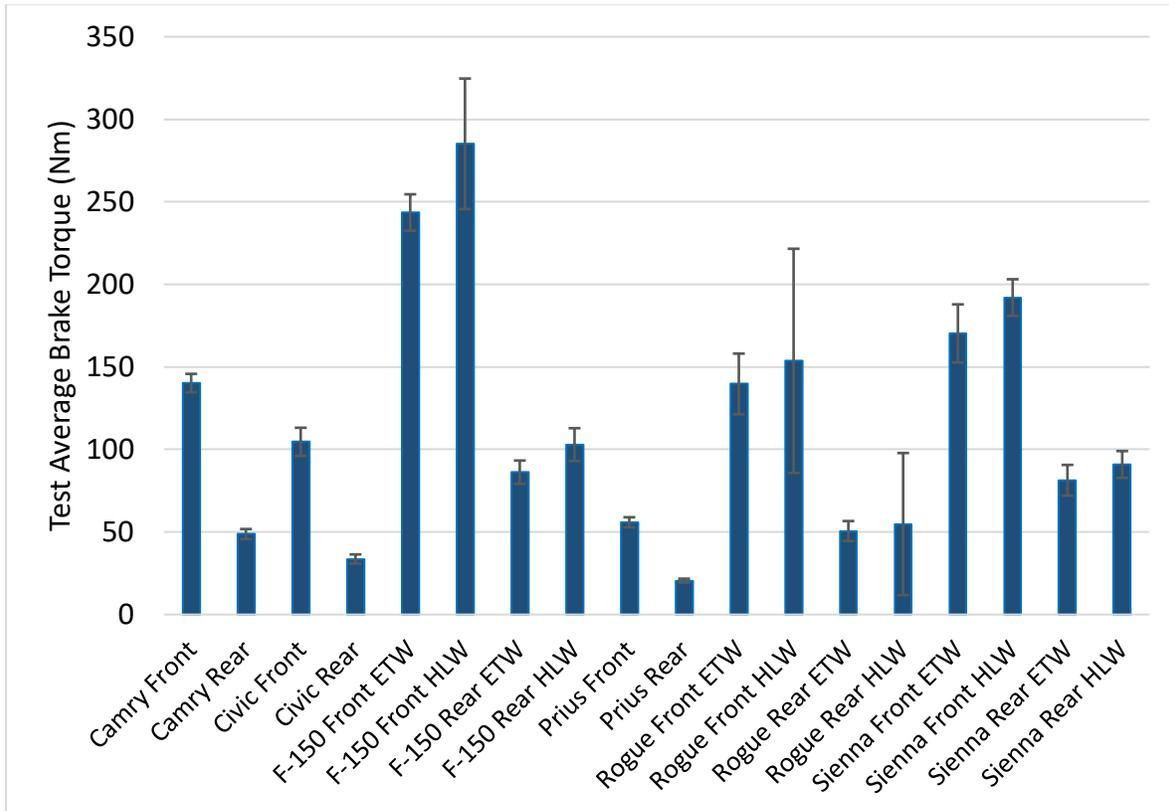
**Figure 39. Average brake torque measured during the CBDC, averaged over all tests of each model, axle, and test weight combination.**
