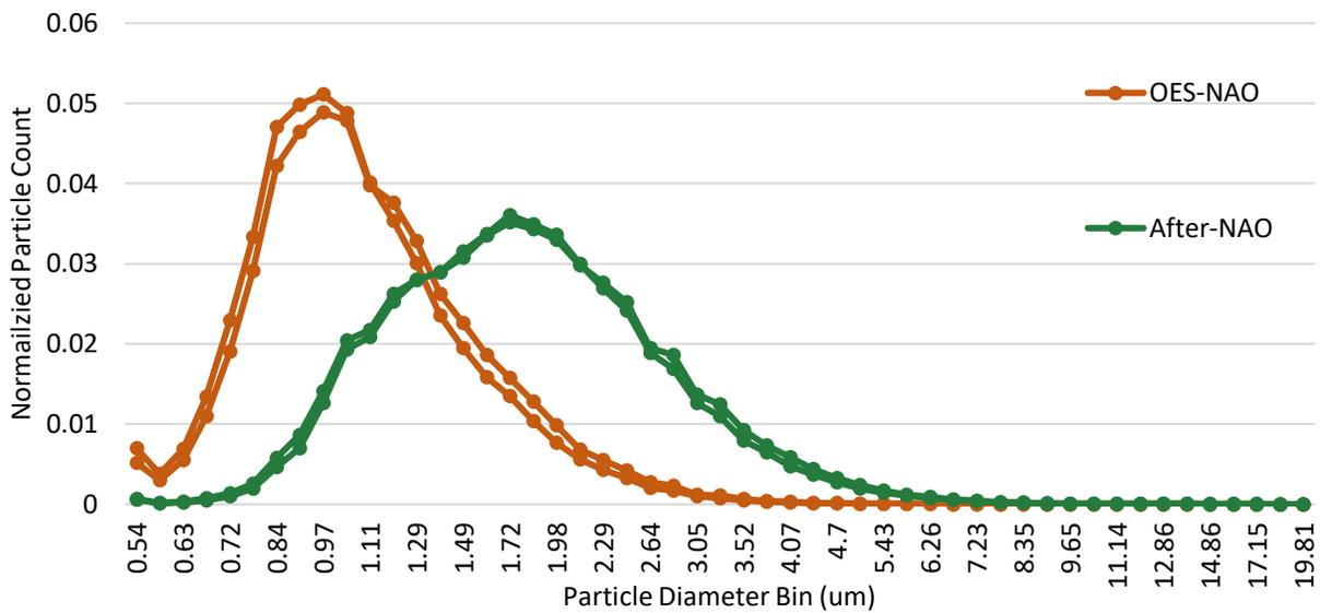
**Figure 64. Size distribution of Civic rear brake PM as measured by APS**
