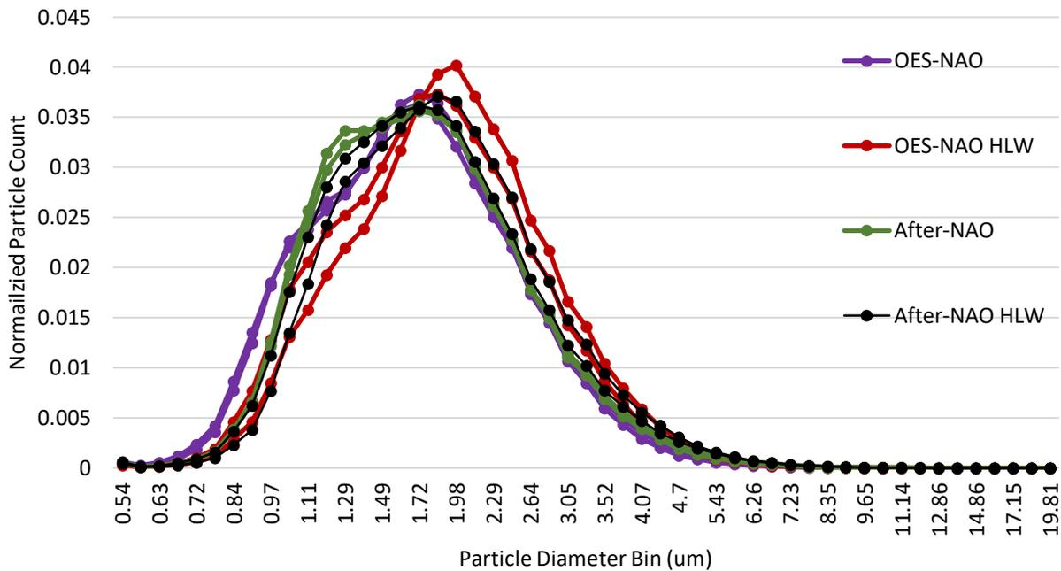
**Figure 71. Size distribution of Sienna front brake PM as measured by APS**
