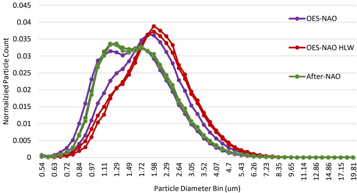
**Figure 69. Size distribution of Rogue front brake PM as measured by APS**
