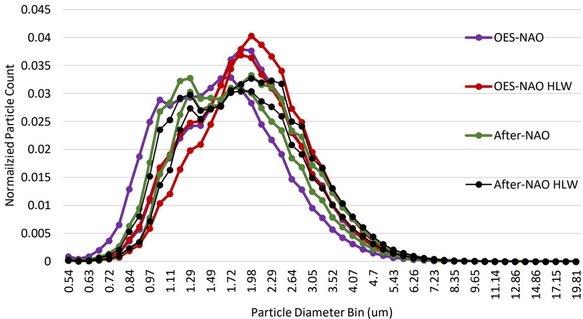
**Figure 72. Size distribution of Sienna rear brake PM as measured by APS**
