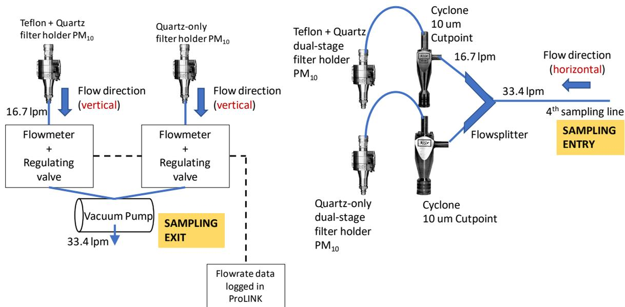
**Figure 30. Detail schematic of Sample Line 4**
