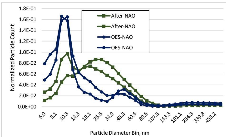
**Figure ES-3. Particle size distribution for the Camry Front axle tests, 5.6-560 nm.**
