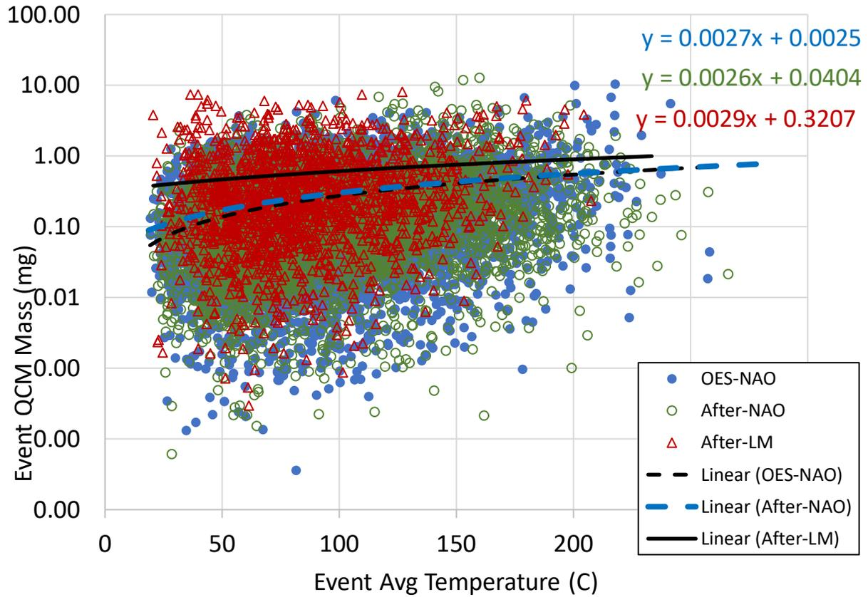
**Figure 77. Trends in QCM brake event PM mass against braking event average rotor temperature, categorized by friction material**
