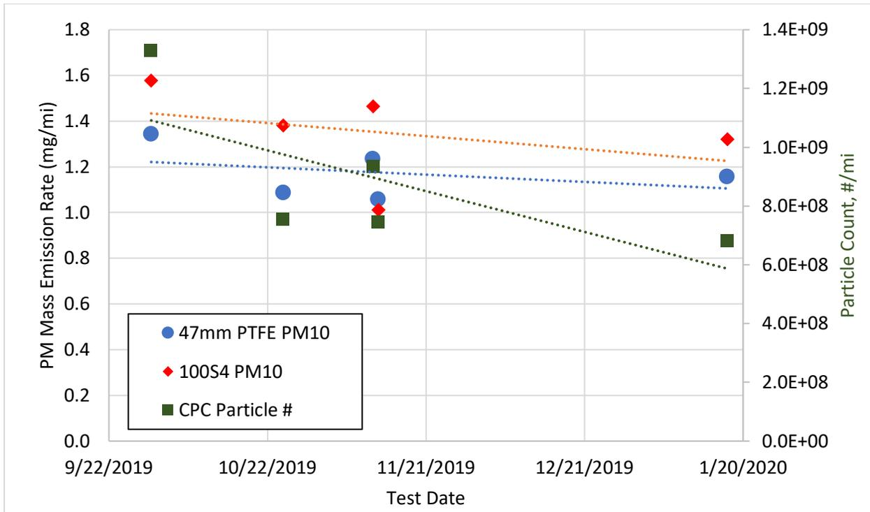
**Figure 95. Reference trends by date for the 47mm PTFE and 100S4 PM10 mass measurements (left axis); and CPC particle count (right axis)**
