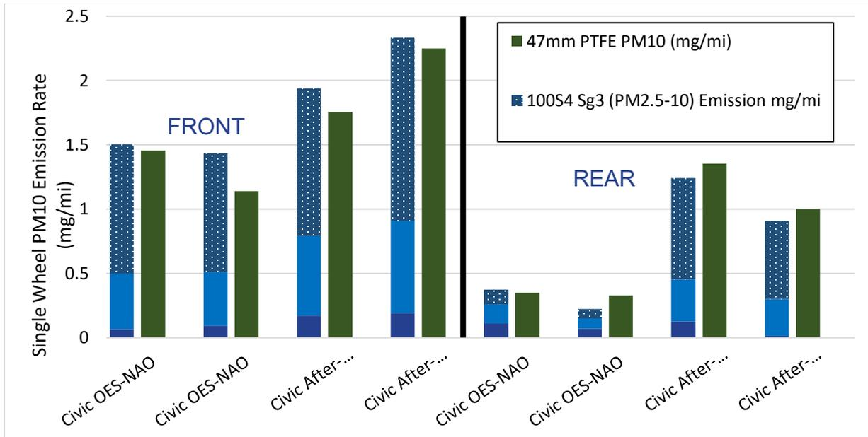
**Figure 41. Single-wheel PM Mass Emission Rates for Civic as measured by 100S4 (Blue) and 47mm Teflon filter (Green). Note the Civic rear brake is a drum system**
