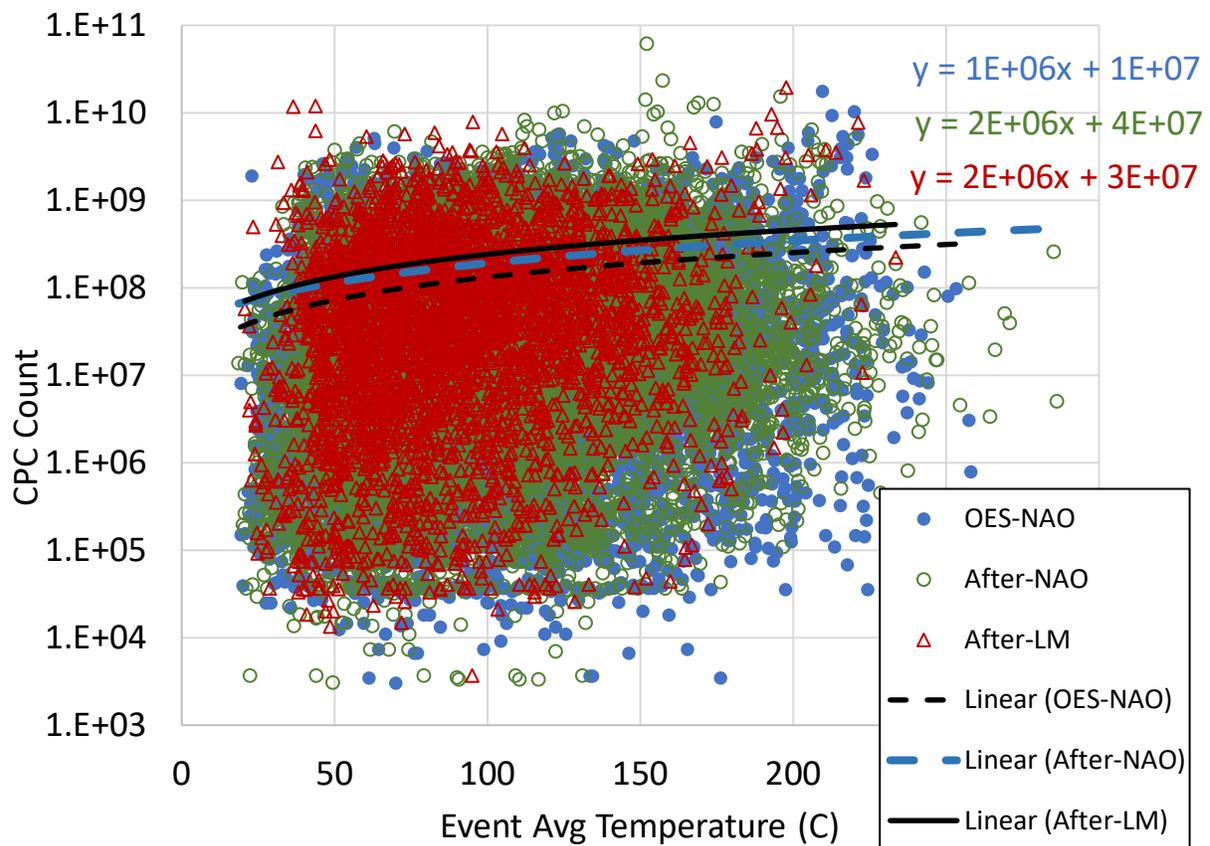
**Figure 76. Trends in total braking event CPC count against average rotor temperature, categorized by friction material**
