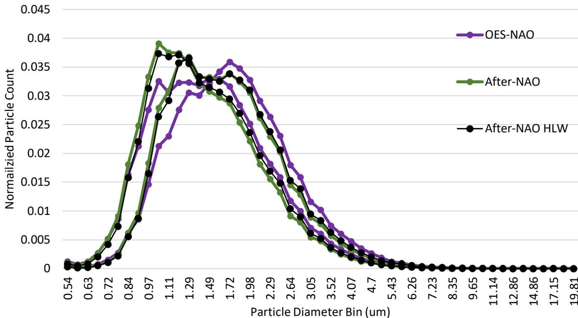
**Figure 70. Size distribution of Rogue rear brake PM as measured by APS**
