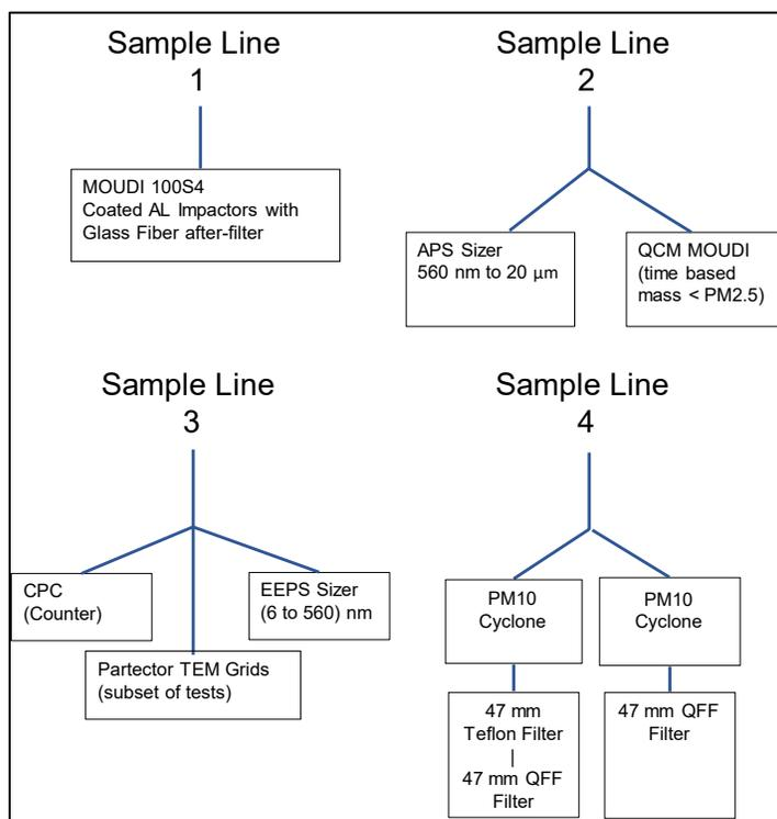
**Figure 29. Sample line schematic for this program**
