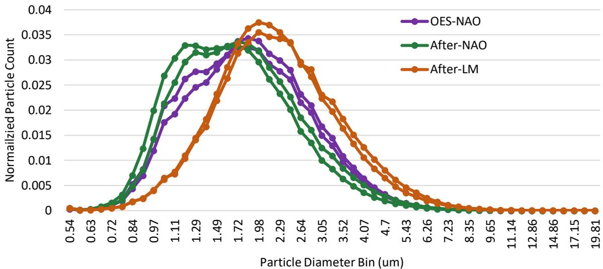
**Figure 61. Size distribution of Camry front brake PM as measured by APS**
