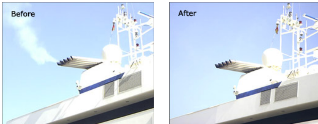
Figure 30. Before and after comparison for MES Super Yacht EcoSilencer
