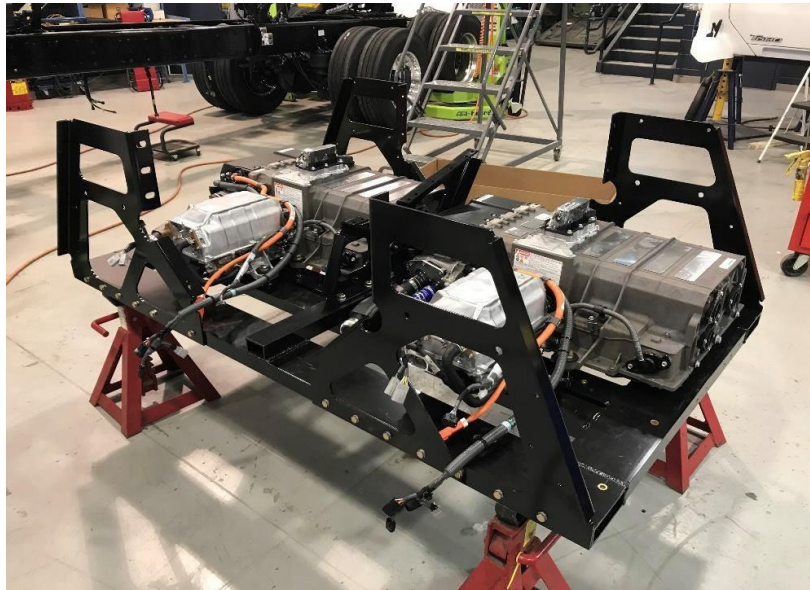
Figure 5. Dual Fuel Cell Assembly
