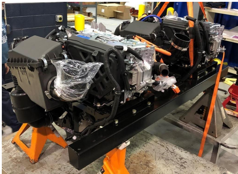
Figure 6. Dual PCU Assembly
