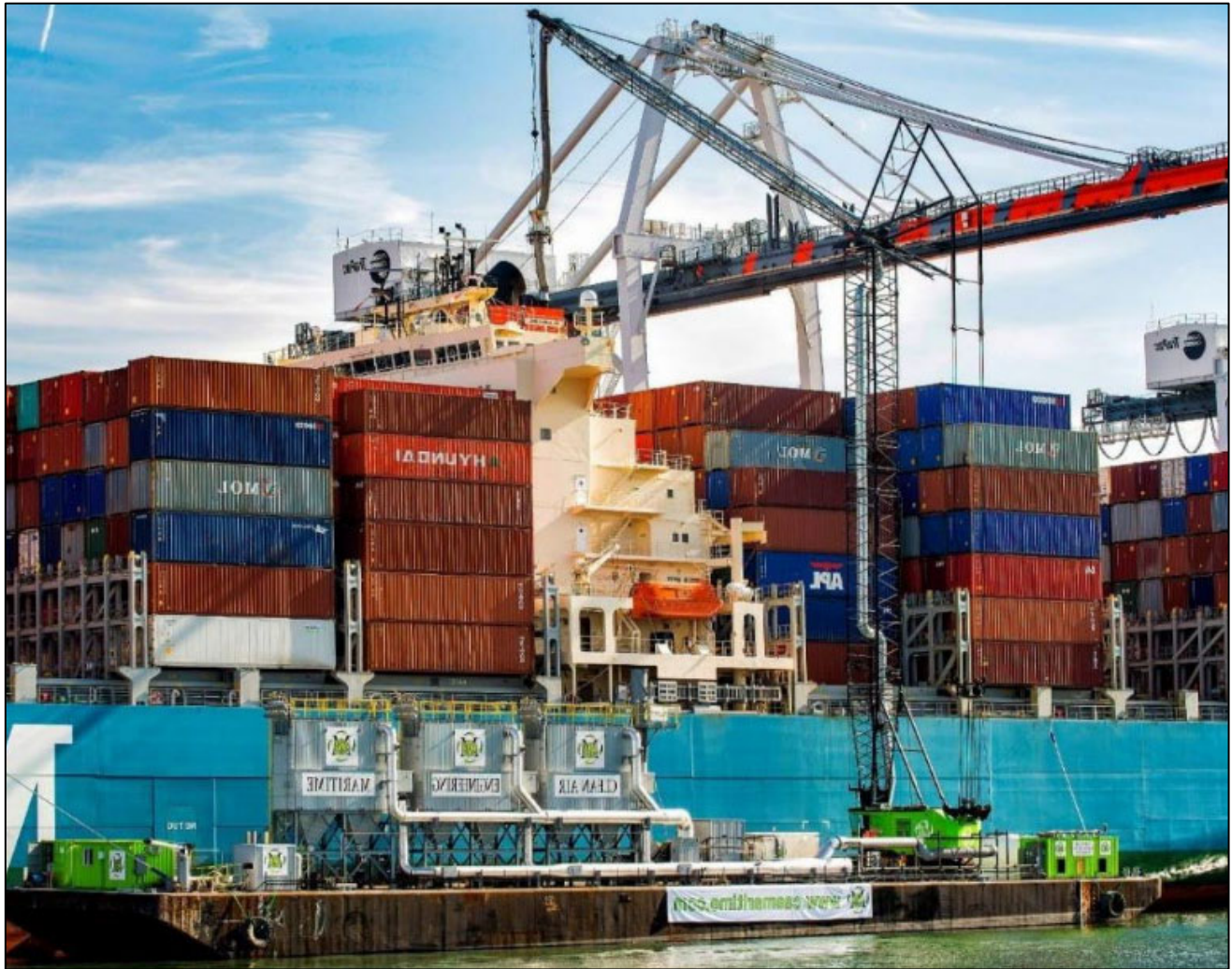
Figure 9: Barge-Based Capture and Control System for Container Vessels (CAEM)
