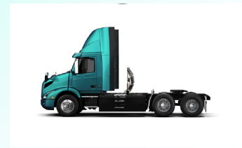
Volvo VNR Electric 175-275 Mi Range Available in 4x2, 6x2 and 6x4 configurations
