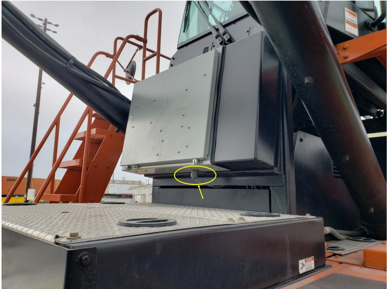
Figure 16. Location Where RPECS Connected to the Electric Side Pick's System CAN Bus
