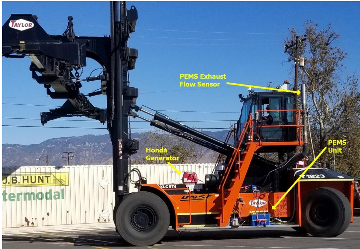
Figure 26. PEMS System Installed on Diesel Side Pick
