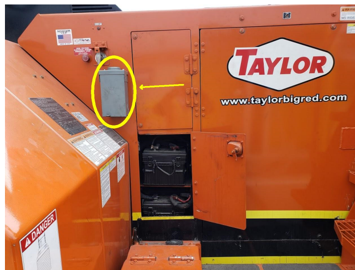
Figure 10. Battery Electric Side Pick Charge Receptacle
