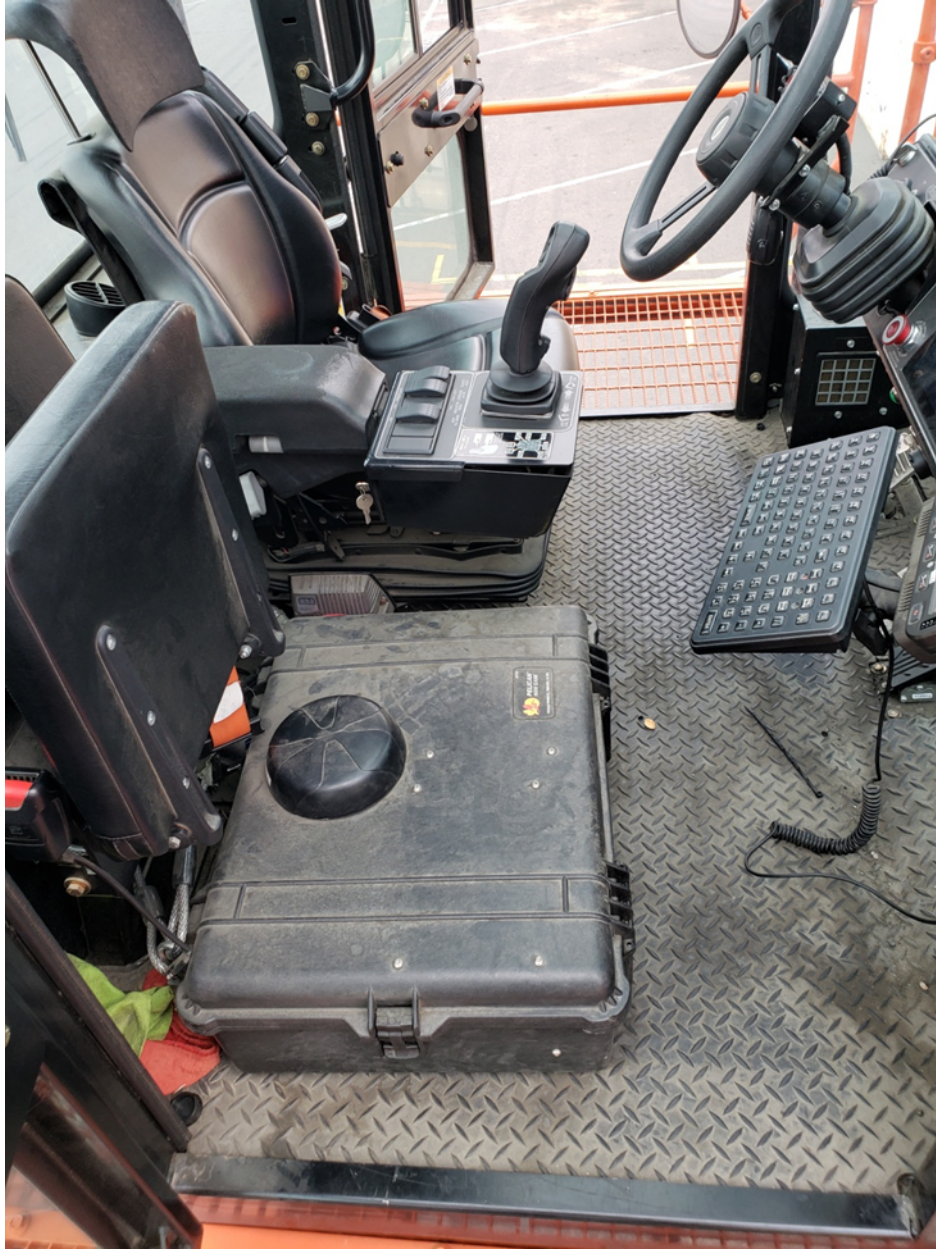
Figure 15. RPECS Datalogger Mounted in the Electric Side Pick Cab
