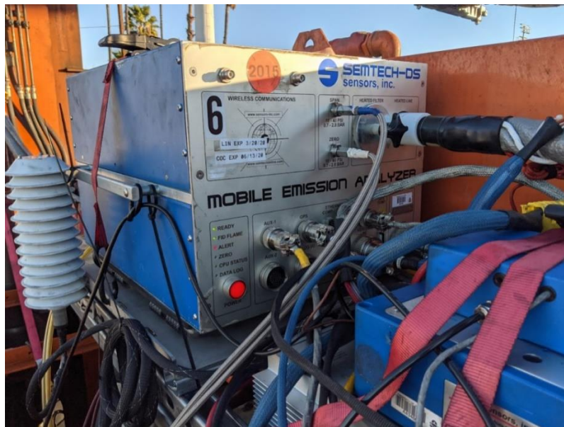
Figure 39. PEMS System Installed on Diesel RTG
