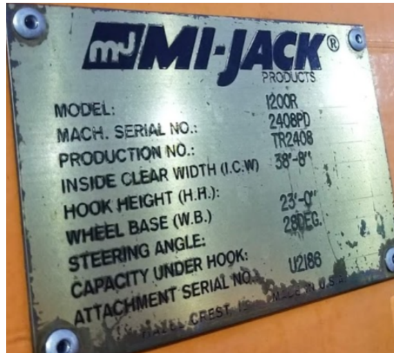
Figure 7. Diesel RTG Information Plate
