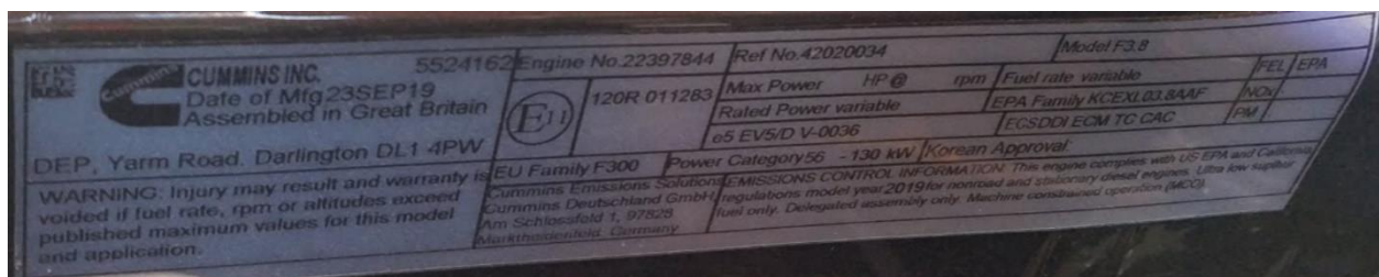
Figure 11. C20 Diesel Engine Data Plate
