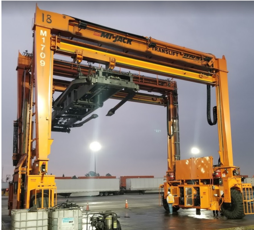
Figure 6. Diesel RTG C18
