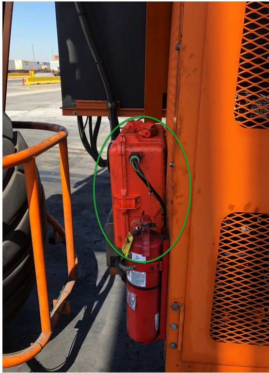
Figure 17. RPECS Datalogger Mounting Locations – Diesel RTG (Left) with RPECS Mounted Outside Engine Compartment and H-RTG (Right) Mounted Inside Electronics Car Body
