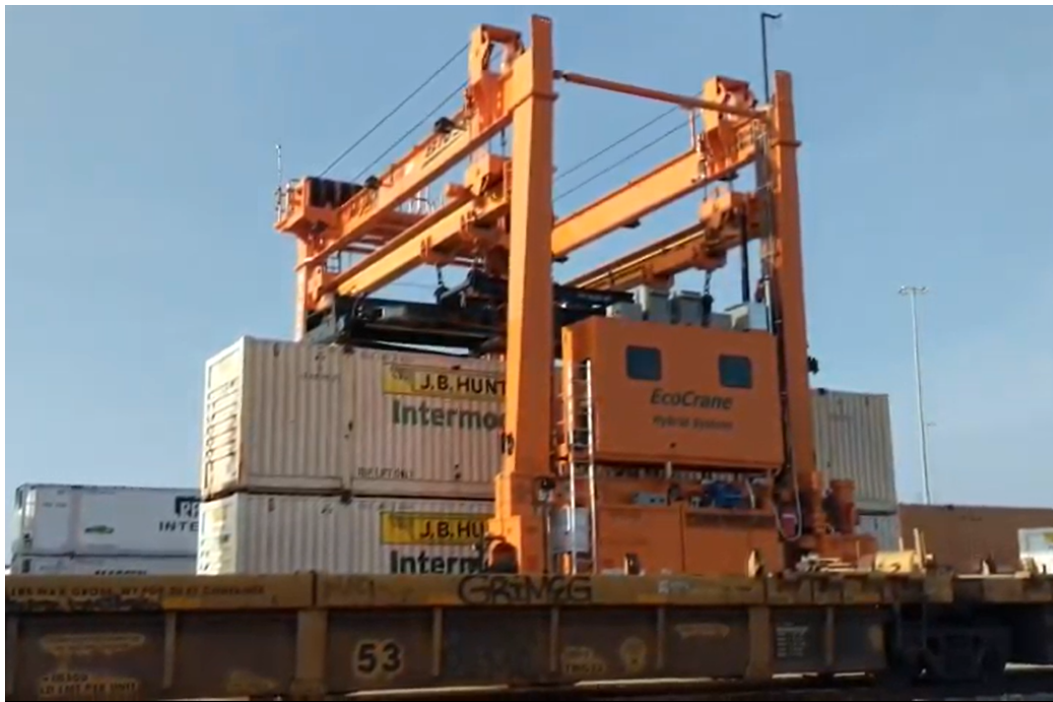
Figure 13. H-RTG Working in BNSF's Stockton Intermodal Yard
