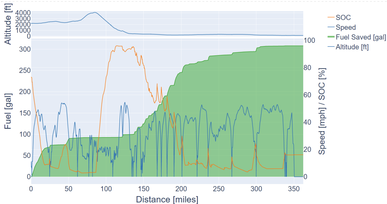
Figure 5 Characteristic Plot Showing Altitude, SOC, Speed, and Estimated Fuel Reduction for a run Traveling from Bartow, CA to Stockton, CA
