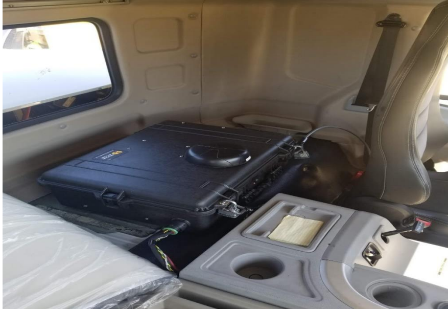
Figure 16. ZANZEFF RPECS Datalogger Mounted in Rear of the BYD Drayage Truck Cab
