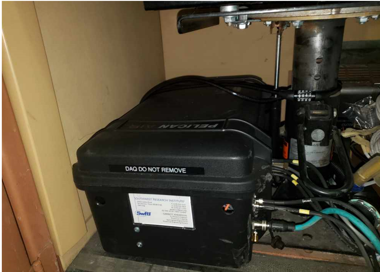
Figure 9. Data Acquisition System Installed on BNSF 3965
