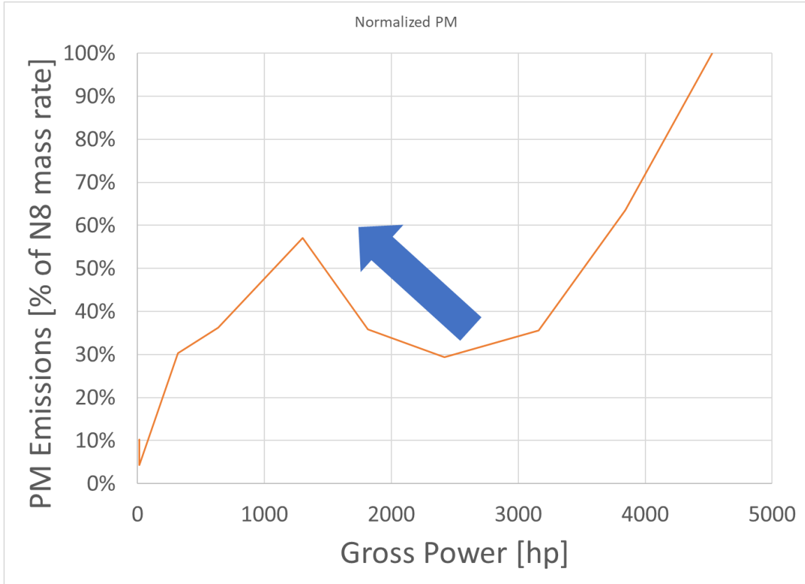
Figure 39. General Trend of PM Rate and BSPM vs Gross Power
