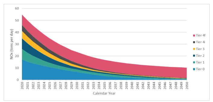
Figure 19. Baseline Statewide NOx emissions by Engine Tier
