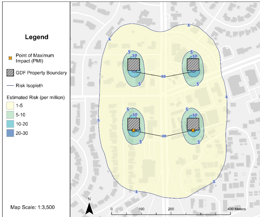
Figure A15. Zone of Impact of Gas Station Emissions: Four Three-Million-Gallon Gas Stations with 200m Separation (Rural) 1,2
