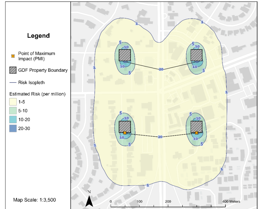
Figure A16. Zone of Impact of Gas Station Emissions: Four Three-Million-Gallon Gas Stations with 250m Separation (Rural) 1,2
