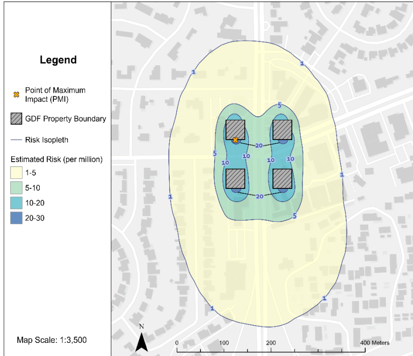
Figure A13. Zone of Impact of Gas Station Emissions: Four Three-Million-Gallon Gas Stations with 100m Separation (Rural) 1,2
