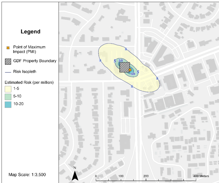
Figure 1. Zone of Impact of Gas Station Emissions: Single Three-Million-Gallon Gas Station (Urban)
