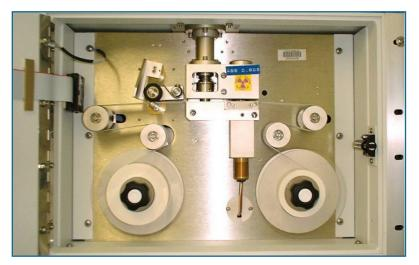
Figure 2. Beta Attenuation Monitor
