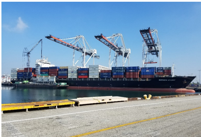
Vessel at berth with a capture and control barge attached to it
