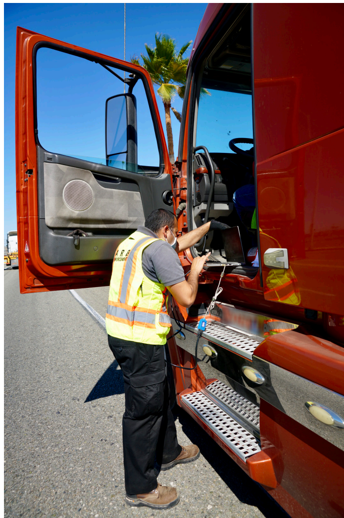
CARB Enforcement staff reading OBD data during a roadside inspection
