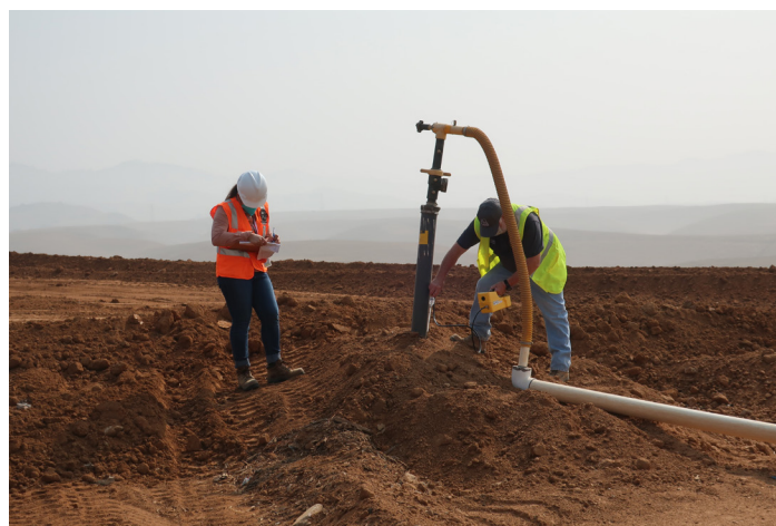
CARB inspectors detecting methane at a landfill gas collection well
