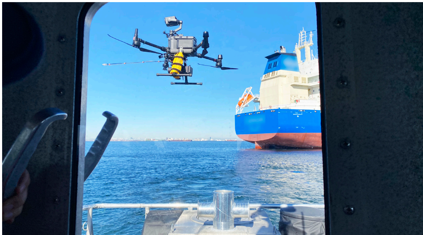
Drone used to analyze ocean-going vessel emissions while at-anchor and underway
