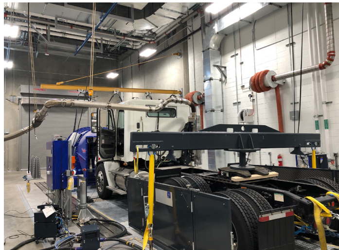
Truck being prepared for in-use compliance chassis testing
