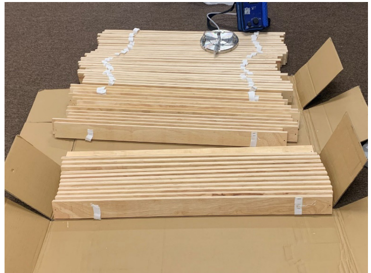
The FLEC screening tool with composite wood products for testing
