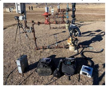
Figure 30: HFS units at METEC. Left to right: Sensors, Inc. (gas sensor module, handheld unit attached by cord), Bacharach HI FLOW, Hetek Flow Sampler, and the AddGlobe GFM.
