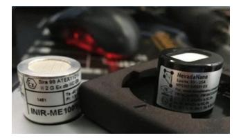
Figure 16: The SGX INIR-ME100 and Nevada Nano MPS Flammable Gas Sensor were chosen for use in the prototype OS-HFS.
