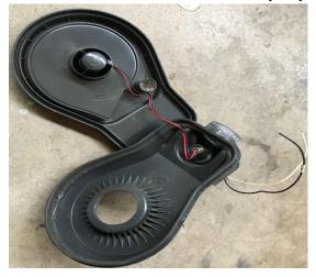
Figure 12: Inside the 3M GVP-100 blower motor used in the BHFS. The blower is certified for use in hazardous areas. All the internal electrical connections are encapsulated. The internal housing (upper left) is characteristic of a centrifugal blower design.
