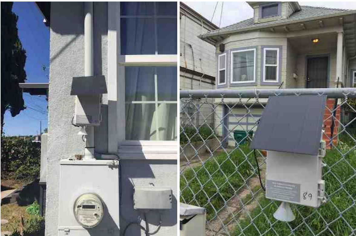
Aerosol Black Carbon Detectors Installed in West Oakland. As depicted here, ABCDs can be installed on fences, poles, and sides of buildings with minimal impact.
