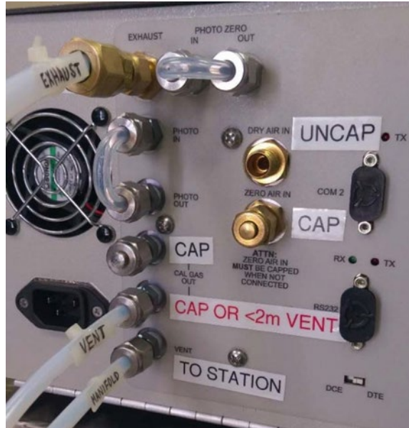
Figure 5: Example Tubing Configuration for Station Manifold Connection - 1/4" OD Tubing to Station Manifold and Second 1/4" Tubing for Venting
