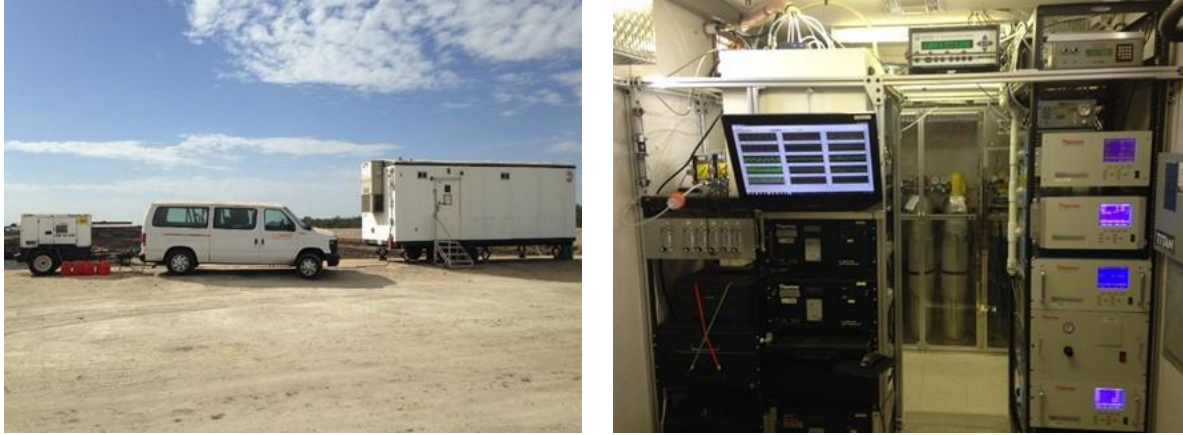
Figure 6. (A) The Mobile Air Quality Laboratory (MAQ Lab) and engine-generator set; (B) different analyzers and supporting equipment onboard of the MAQ Lab.
