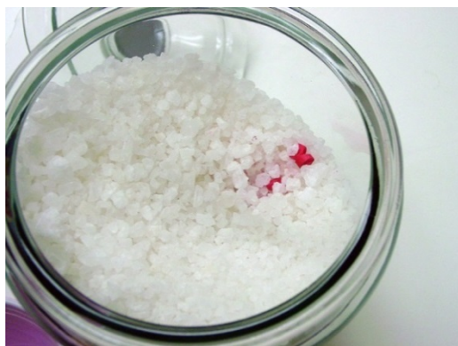
A. Crushed salt and red chalk (spike) before pulverization.
