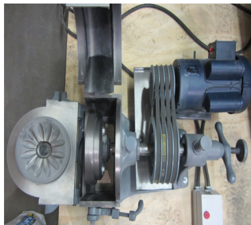
B. Plate grinder for pulverization.
