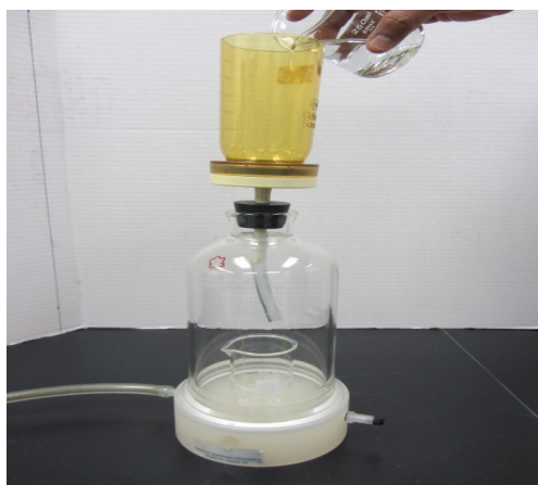
B. Suction filtration of acid digest.
