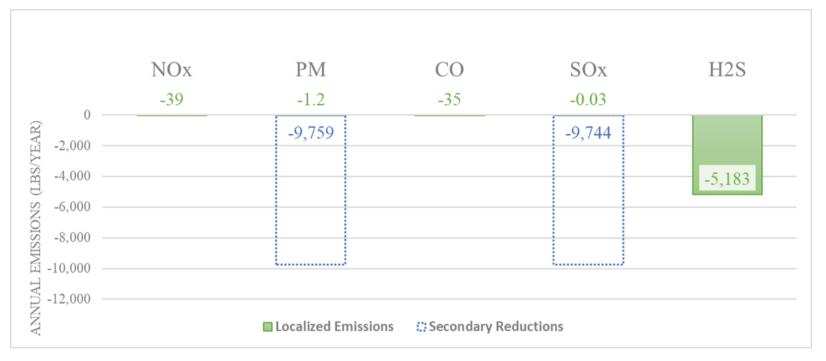
"Localized" refers to emissions that occur at the dairy. "Secondary" refers to reductions in H2S that in turn reduce sulfate particles in the atmosphere (H2S oxidizes into SOx; SOx participates in the formation of PM).
