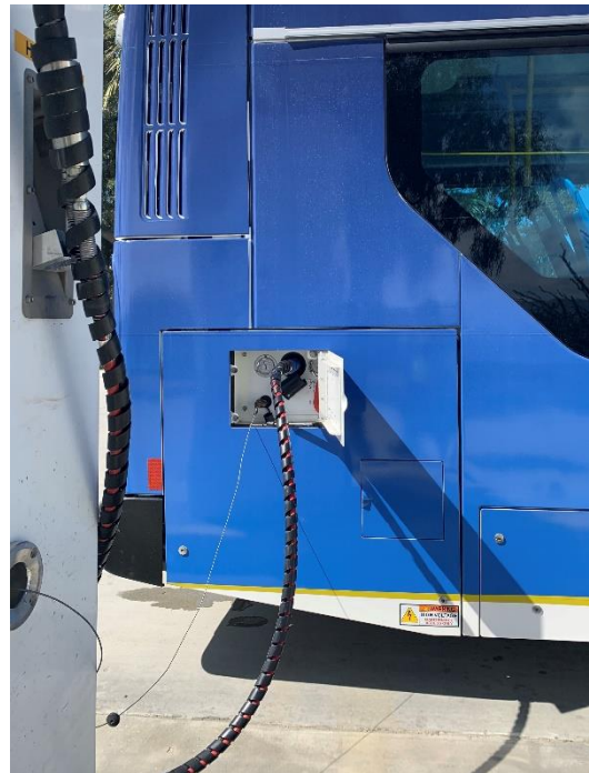
Photo 2: Fuel Cell Energy Bus Refueling
