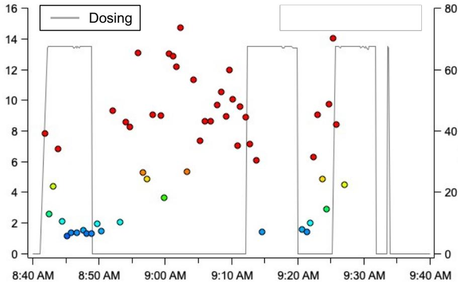
Time series of the urea dosing rate (grey line) and the corresponding NO<sub>x</sub> emission factors measured at the exhaust tailpipe for engine condition 17. The SCR system was not dosing consistently. Emission factors are high when dosing is stopped, and these high emission factors occurred during slow cruise, maneuvering, and docked operating modes (Figure 52).
