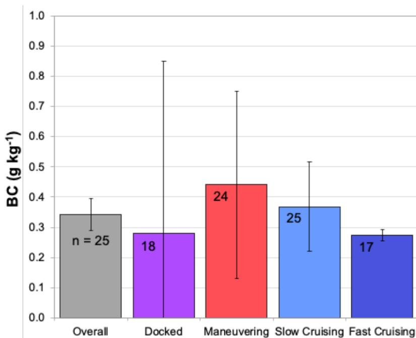
The overall and mode-specific average BC emission factors for the sampled fleet of ferry and excursion vessels. The number (n) of engine conditions included in each average value is noted in each bar. The error bars represent 95% confidence intervals about these arithmetic means. The overall BC emission factor was determined by a weighted average scheme described in the text above.
