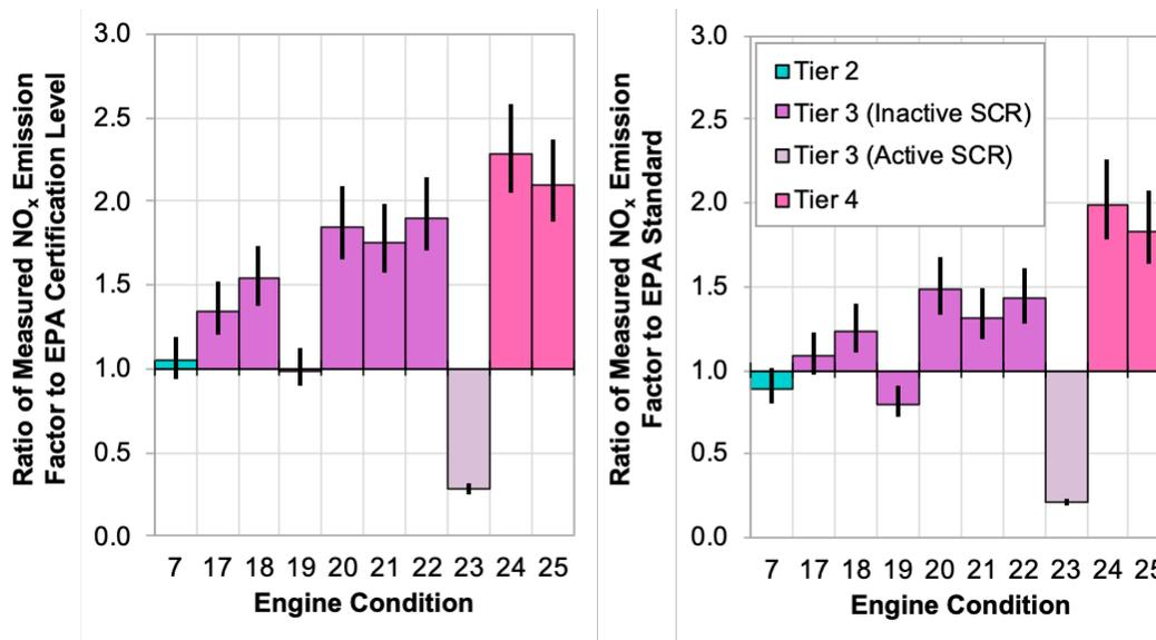
**Ratio of the average NO<sub>x</sub> emission factor measured for each engine condition in this study and the corresponding EPA (a) certification value for that engine and (b) emission standard. Values less than one indicate real-world NO<sub>x</sub> emission rates that meet the certification value or exhaust standard, whereas values greater than one represent measured emissions that exceeded the engine’s certification value or standard.**
