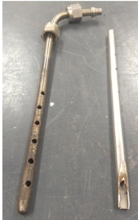
Gaseous probe (left) and PM probe (right).
