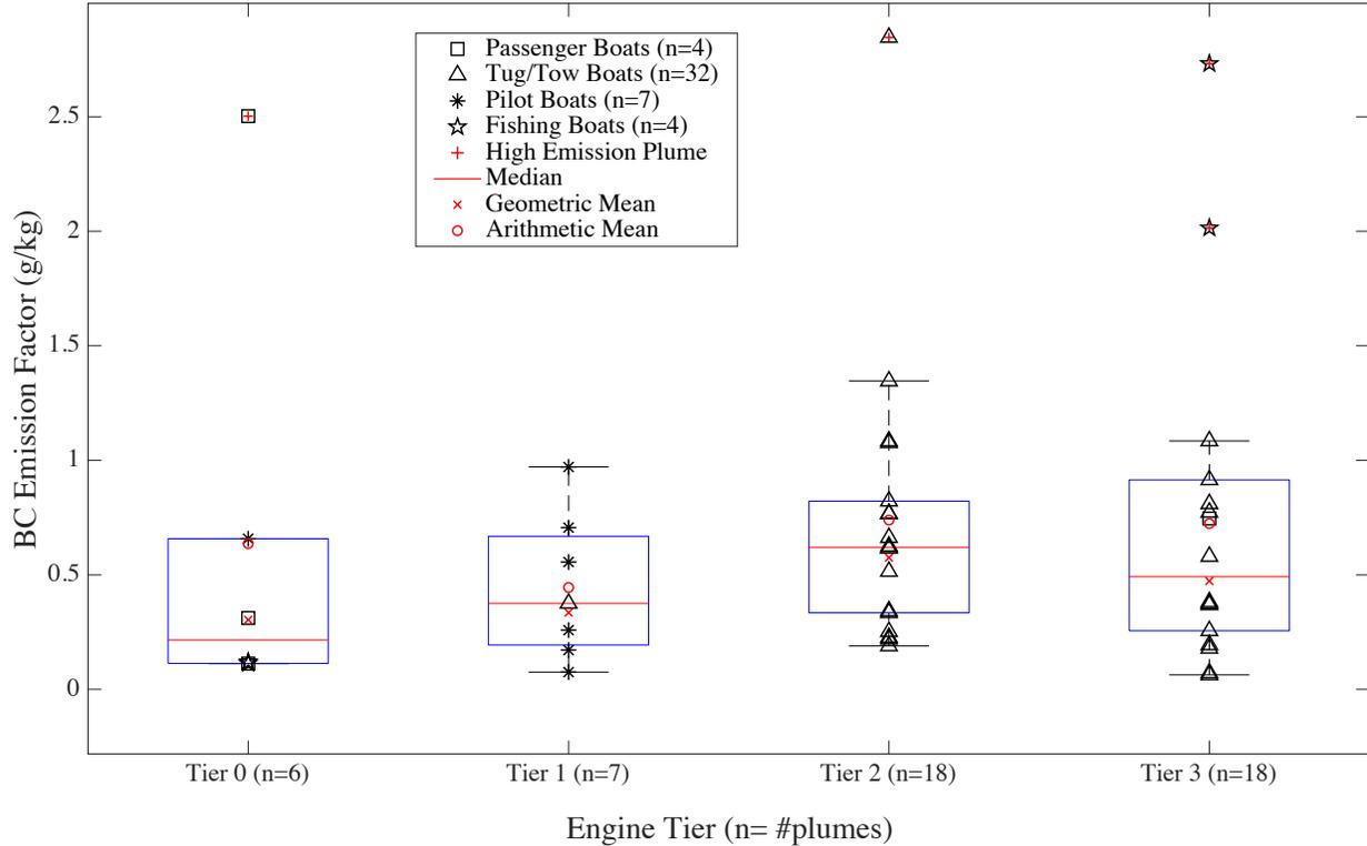
**Boxplots of non-idling onshore measurements of the 27 vessels with engine information provided by CARB. Black symbols indicate vessel types and red symbols indicate statistics.**
