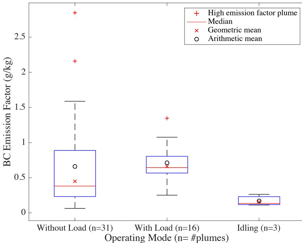
Boxplots of BC emission factors measured from tug and tow boats separated by operating mode. High emission factors are statistical outliers defined as emission factors greater than the 75<sup>th</sup> percentile of emission factors from that operating mode plus 1.5 times the interquartile range.
