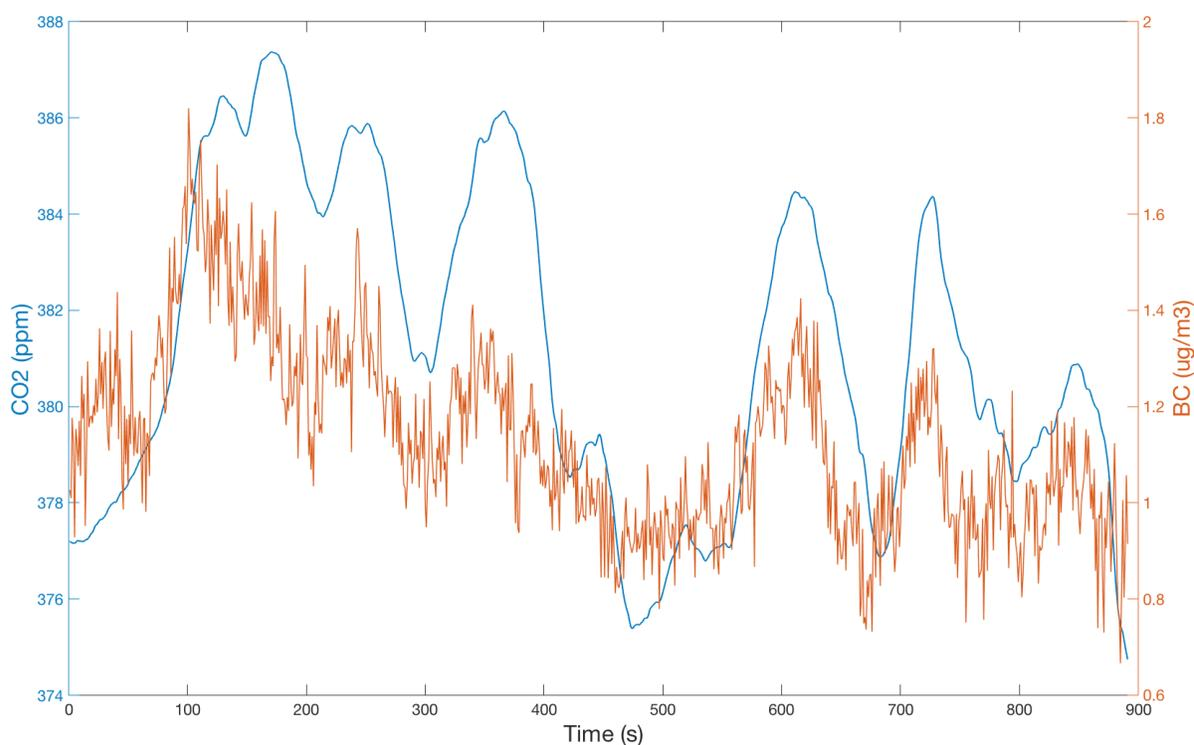
**Plume 4 ABCD data that has been smoothed with a 40-second moving average (orange) and matched to the corresponding CO<sub>2</sub> plume (blue).**
