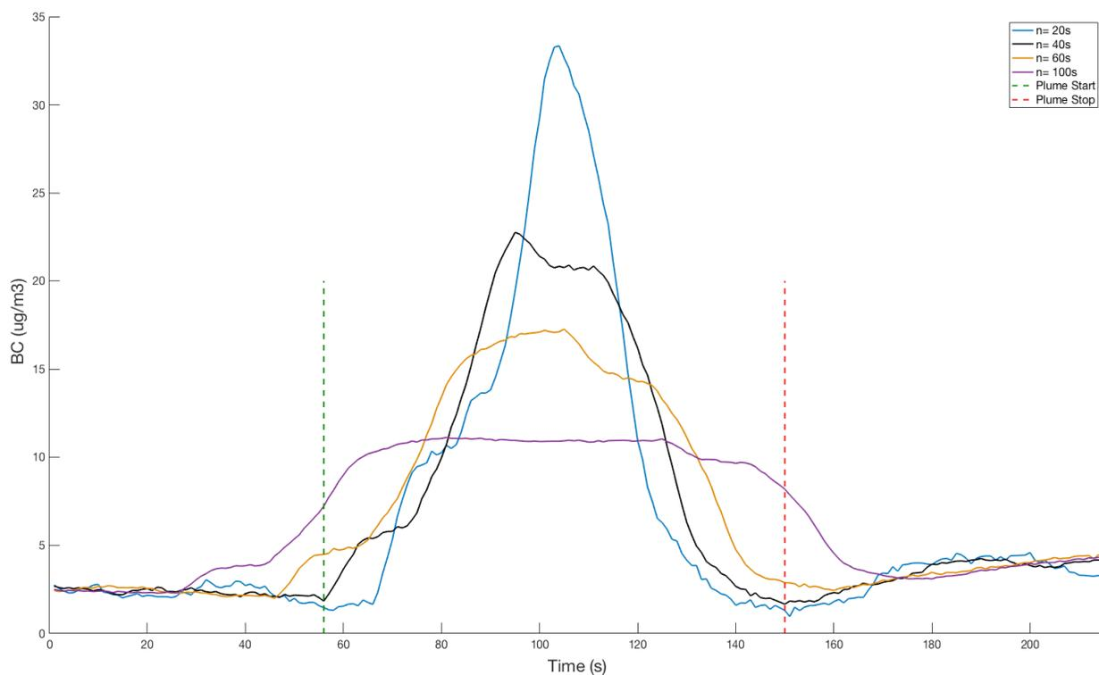
**Comparison of Plume 2 smoothed with different window widths.**
