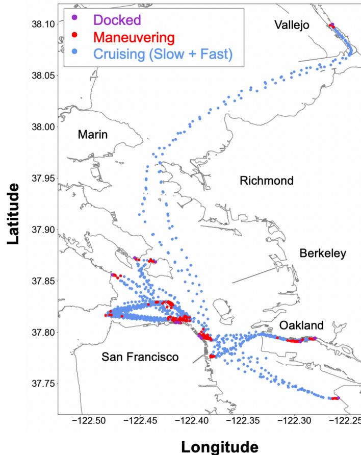
**This map shows 1438 individual plume capture events of 25 engine conditions on 14 ferry and excursion vessels across the San Francisco Bay. Each measurement is categorized by operating mode, based on handwritten field notes and refined by speed data, as described in the text.**
