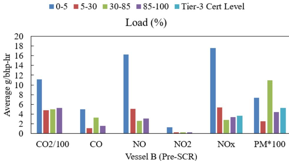
The transient emission data was shown in Figure 26 for Vessel B in the pre-SCR or engine-out sampling position. This was a typical run for the vessel. The overall operational states of the vessel are quite similar to Vessel A. While loading and unloading the vessel is kept in gear to
