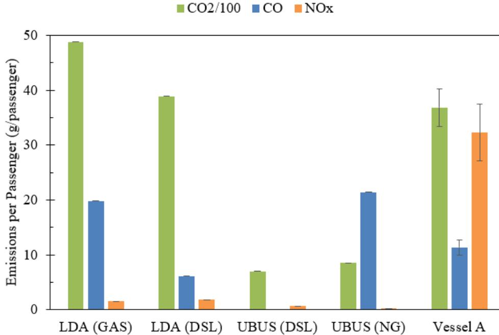
Emission comparison per passenger between the Light Duty Automobile (LDA), Urban Bus (UBUS), and the Vessel A. The LDA is given for gas and diesel fuels. The UBUS is given for diesel and natural gas fuels. Emission data for the vehicles was provided by the EMFAC2017 model.
