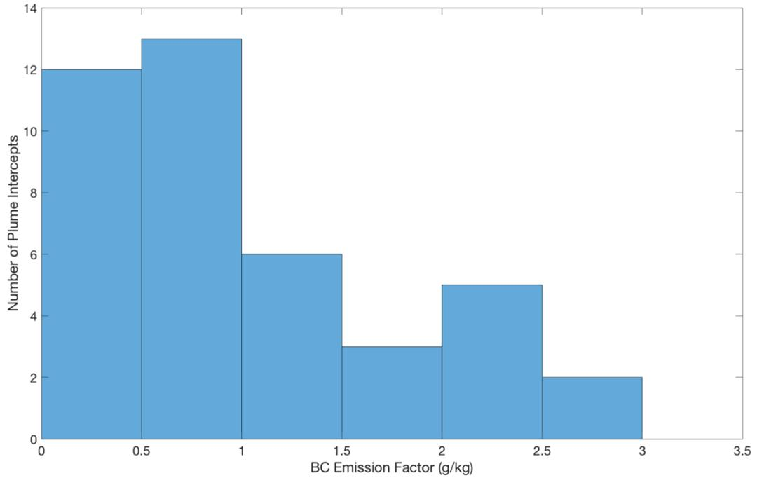
Distribution of BC emission factors (n = 41) measured on-board a Tier 1 fishing boat with dry exhaust.
