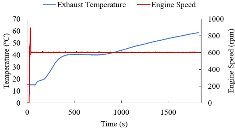
**Engine exhaust temperature as measured in the sample line branched from the exhaust pipe in the post-SCR position.**
