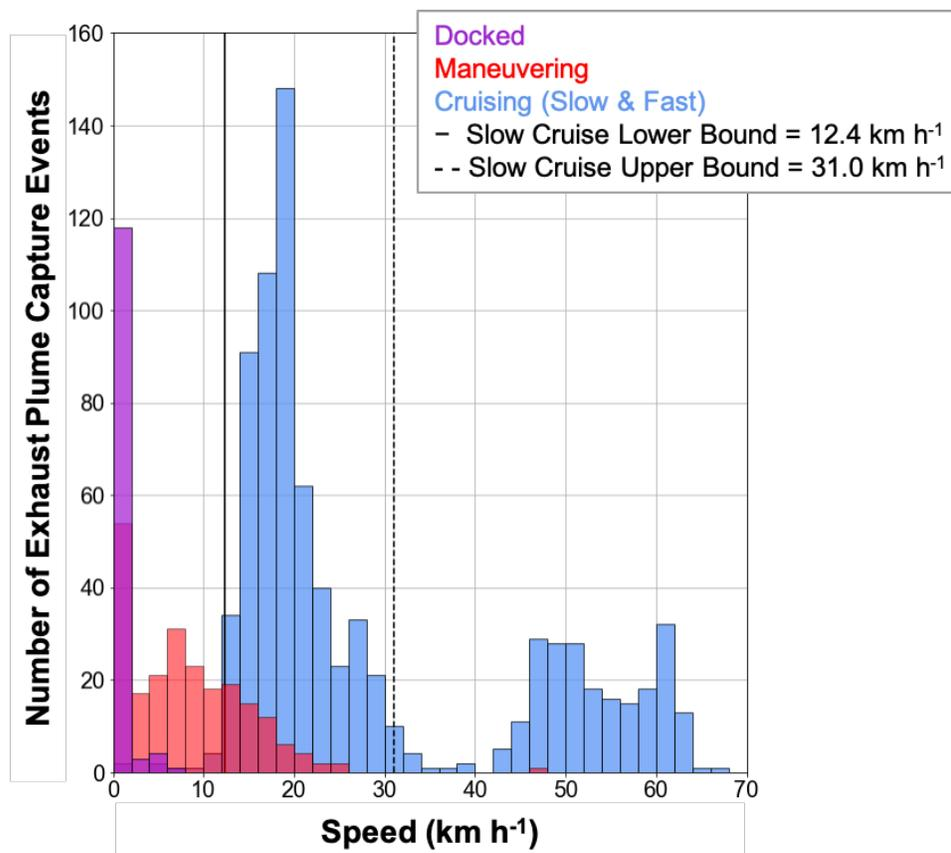
Distribution of vessel speeds during 1438 plume capture events, where each event resulted in a calculated BC emission factor. Each emission factor was categorized by operating mode, as described above in the text.
