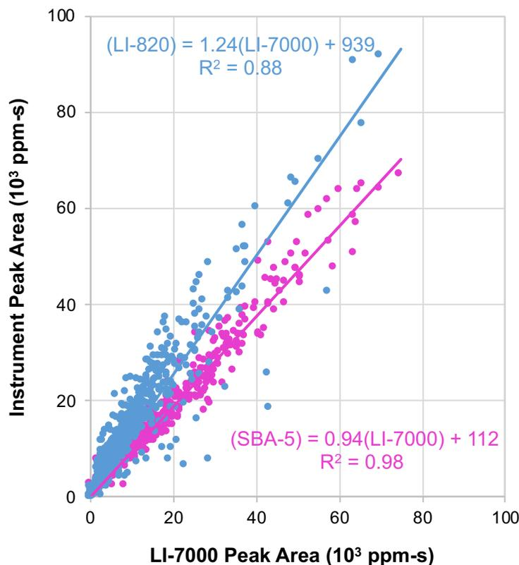
Linear relationships of  $CO_2$  peak areas (ppm-seconds) calculated with the LI-820 and SBA-5 relative to the faster-responding LI-7000 for the same plume capture events measured on-board in-use vessels.
