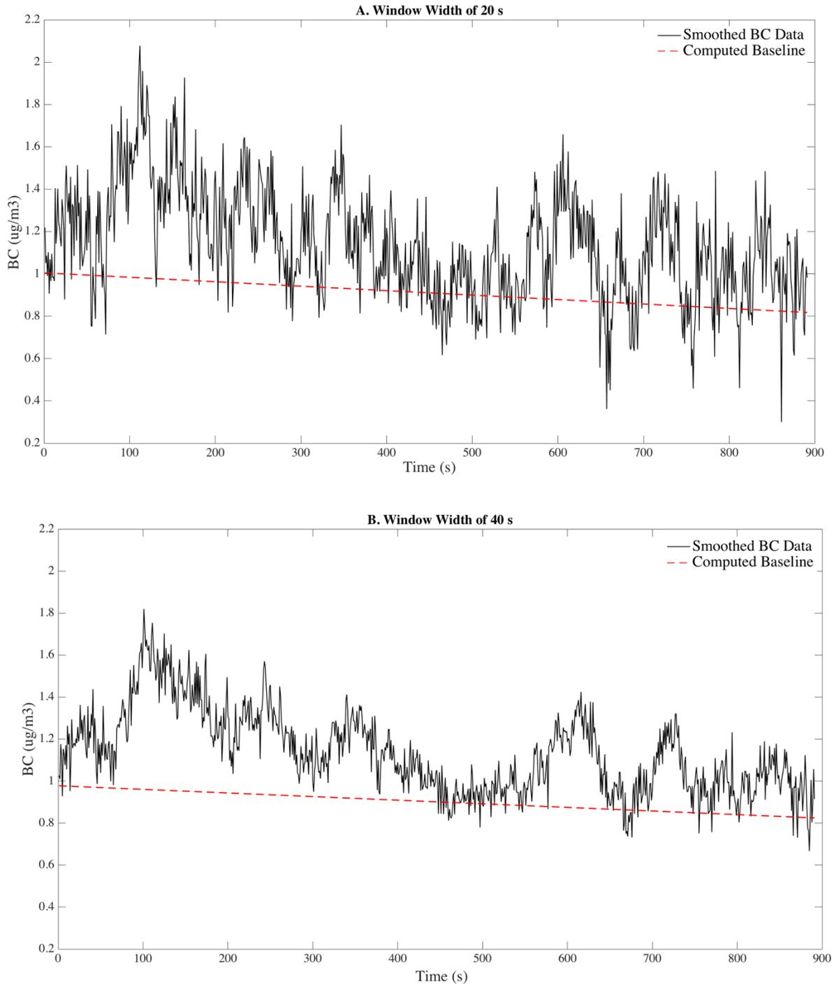
**Comparison of the moving BC baseline (red dashed line) calculated for Plume 4 (black) when data were smoothed using a 20-second moving average (A) versus a 40-second moving average (B).**
