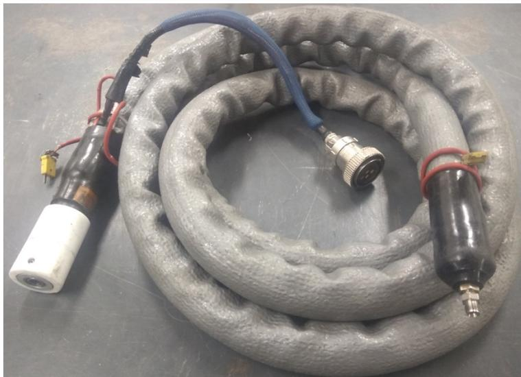
**AVL M.O.V.E heated sample line (top), its extension (middle), and heated sample line for the Sensor SEMTECH (bottom).**
