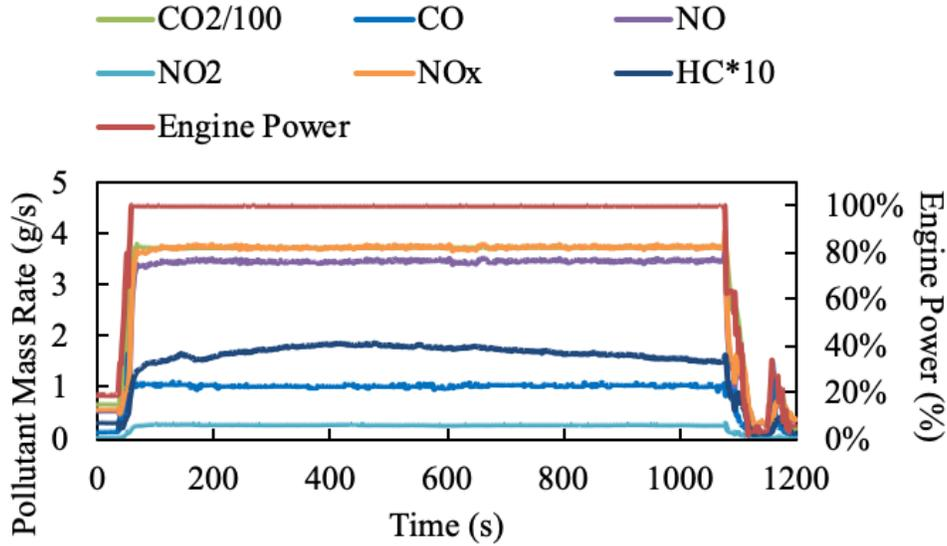
**Time series of emissions for run 3A on 1/22/2019 on Vessel A.**
