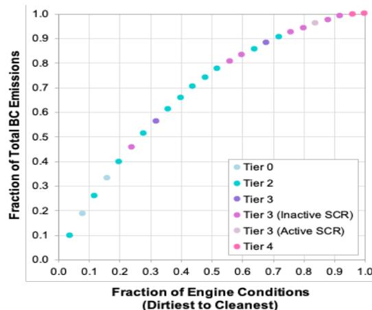
Figure 6 shows the ratio of the overall BC emission factor measured for each engine condition and corresponding U.S. EPA engine
