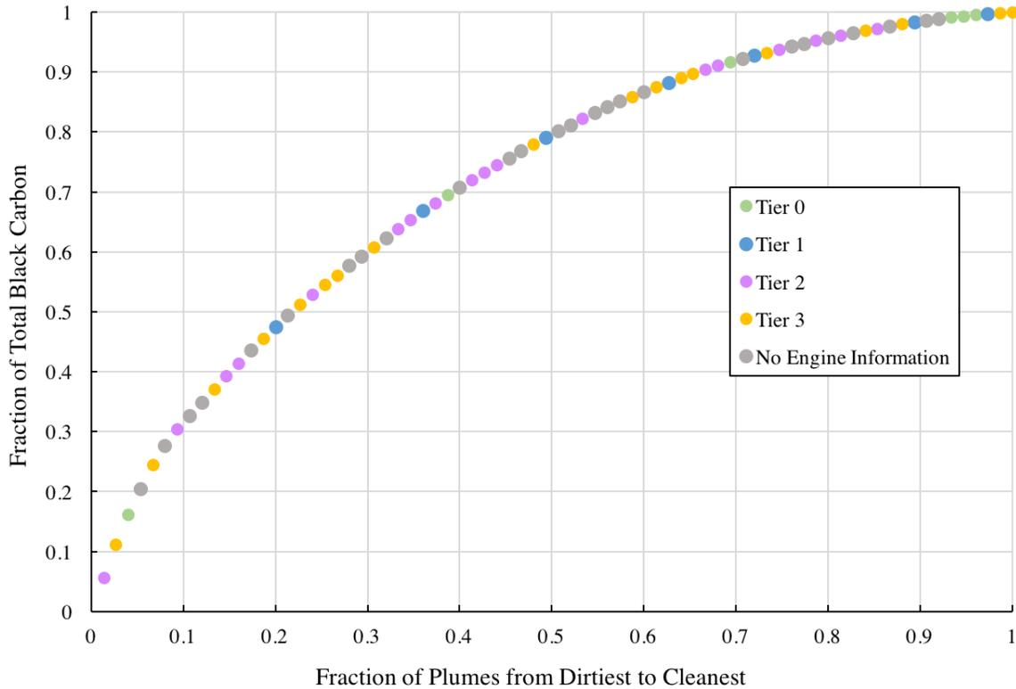
**Cumulative BC emission factor distribution of onshore measurements with EPA engine tiers labelled when available.**
