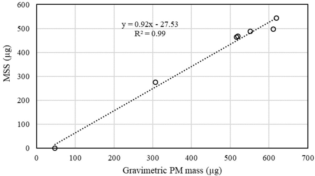
Comparison of PM mass measured by gravimetric method and MSS for Vessel B.
