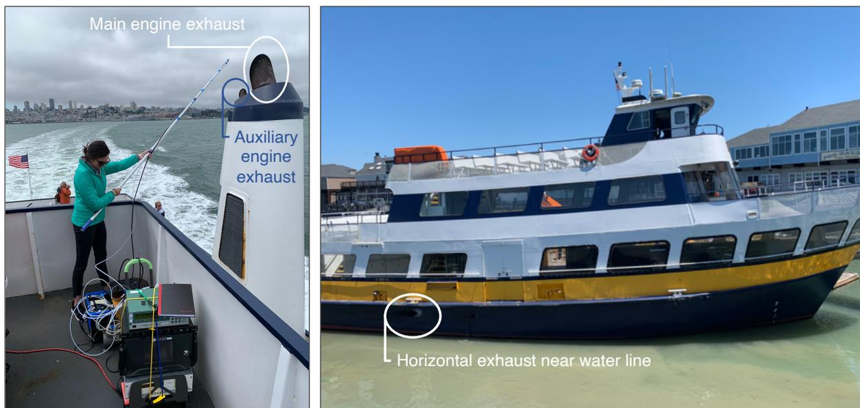
**(Left) Vertically-oriented exhaust, with auxiliary engine exhaust adjacent to the main engine exhaust tailpipe. The gas and particle sample lines are attached to the pole, which is extended intermittently into the main engine exhaust plume. (Right) Horizontally-oriented main engine exhaust.**
