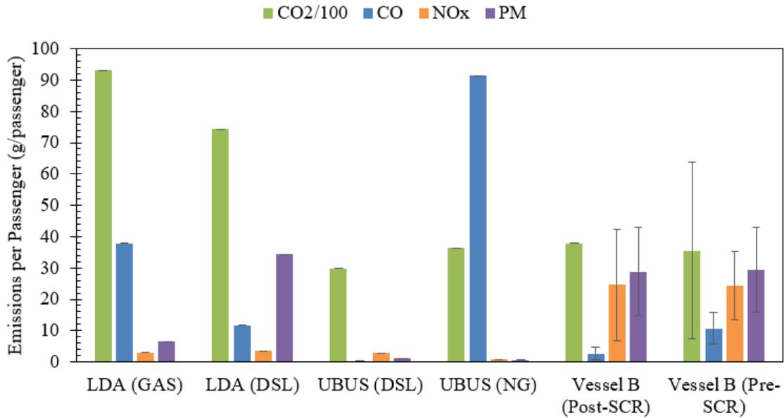
Emission comparison per passenger between the Light Duty Automobile (LDA), Urban Bus (UBUS), and the Vessel B for both sampling positions. The LDA is given for gas and diesel fuels. The UBUS is given for diesel and natural gas fuels. Emission data for the vehicles was provided by the EMFAC2017 model.
