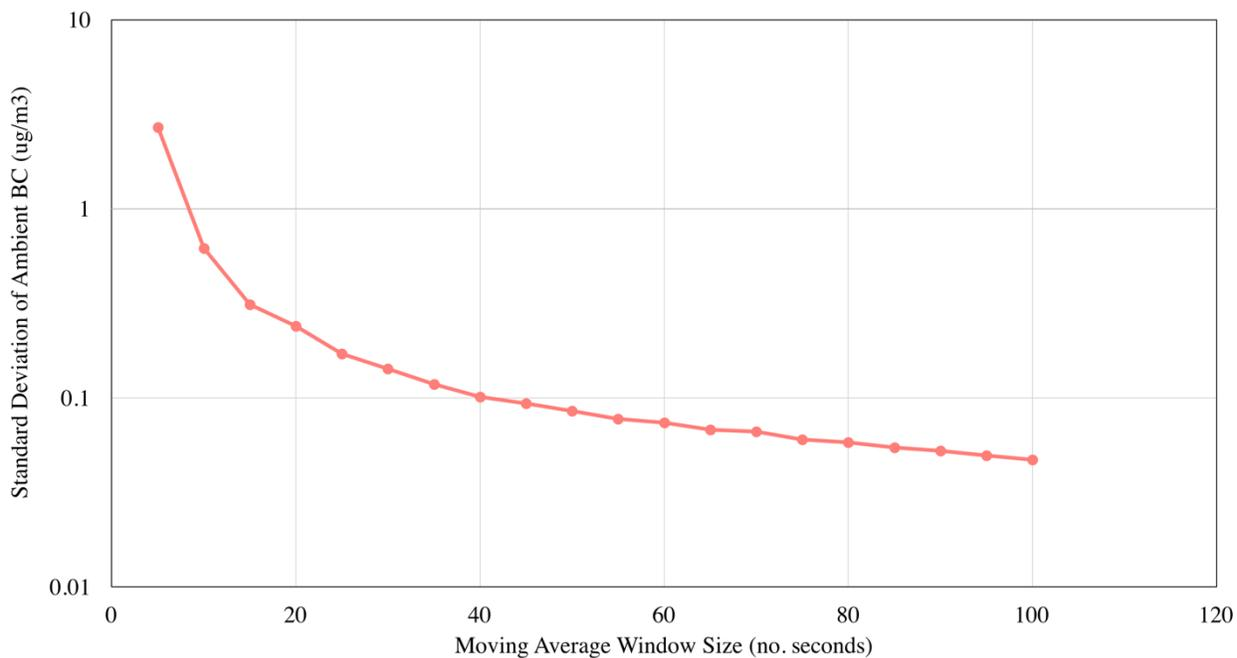
Noise observed in 200 seconds of ABCD measurements of ambient BC after smoothing data with different window widths.
