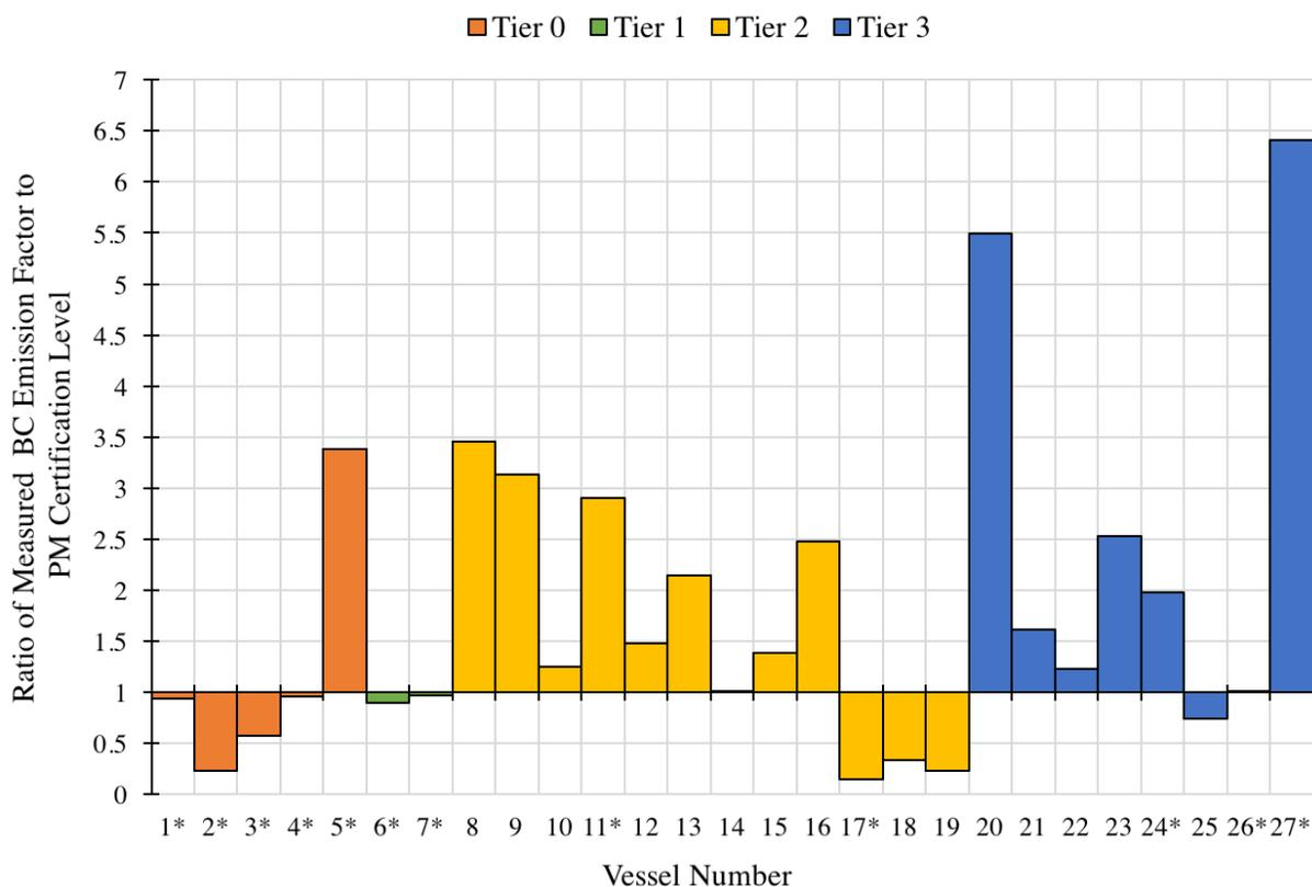
EPA PM certification levels were provided by CARB when available and estimated from CARB’s emission inventory (denoted by asterisks) when engine information was missing. These data were compared to the arithmetic mean of non-idling BC emission factors. Ratios greater than 1 indicate vessels with average BC emission factors that are greater than their PM certification level and ratios less than 1 indicate vessels with average BC emission factors lower than their PM certification level.
