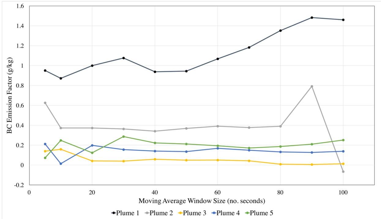
**BC emission factors for five different plumes that were computed using smoothed data with varying window widths. The moving average window size corresponds to the number of data points used to smooth the BC data.**
