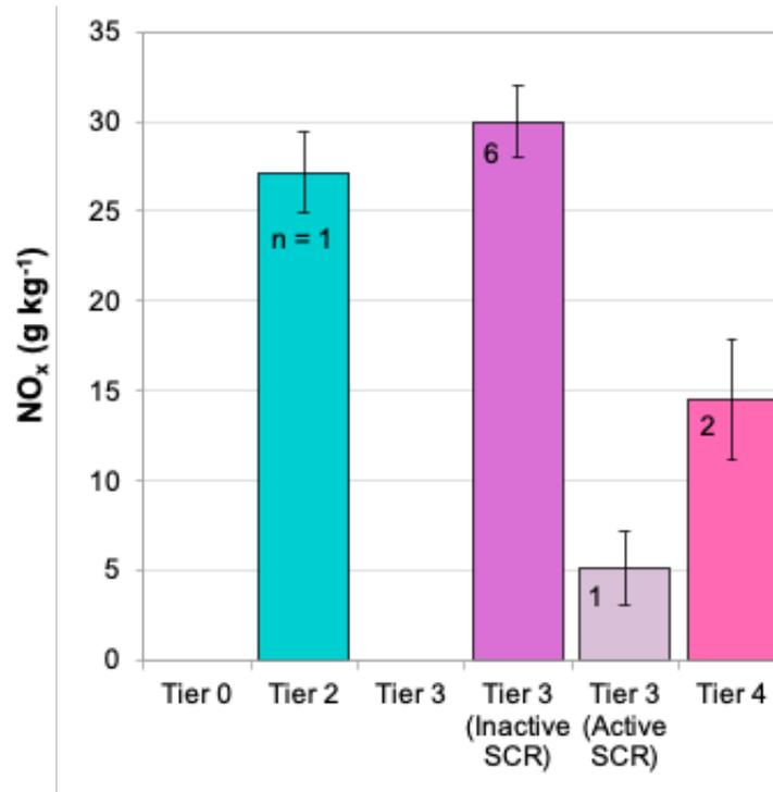
Overall NO<sub>x</sub> emission factors ( $\pm 95\%$  confidence interval) by engine tier, based on the subset of 10 engine conditions with NO<sub>x</sub> measurements and as also summarized in Table 13. The number (n) of engine conditions included in each average value is noted in each bar. The overall NO<sub>x</sub> emission factor was determined by a weighted average scheme described in the text above.
