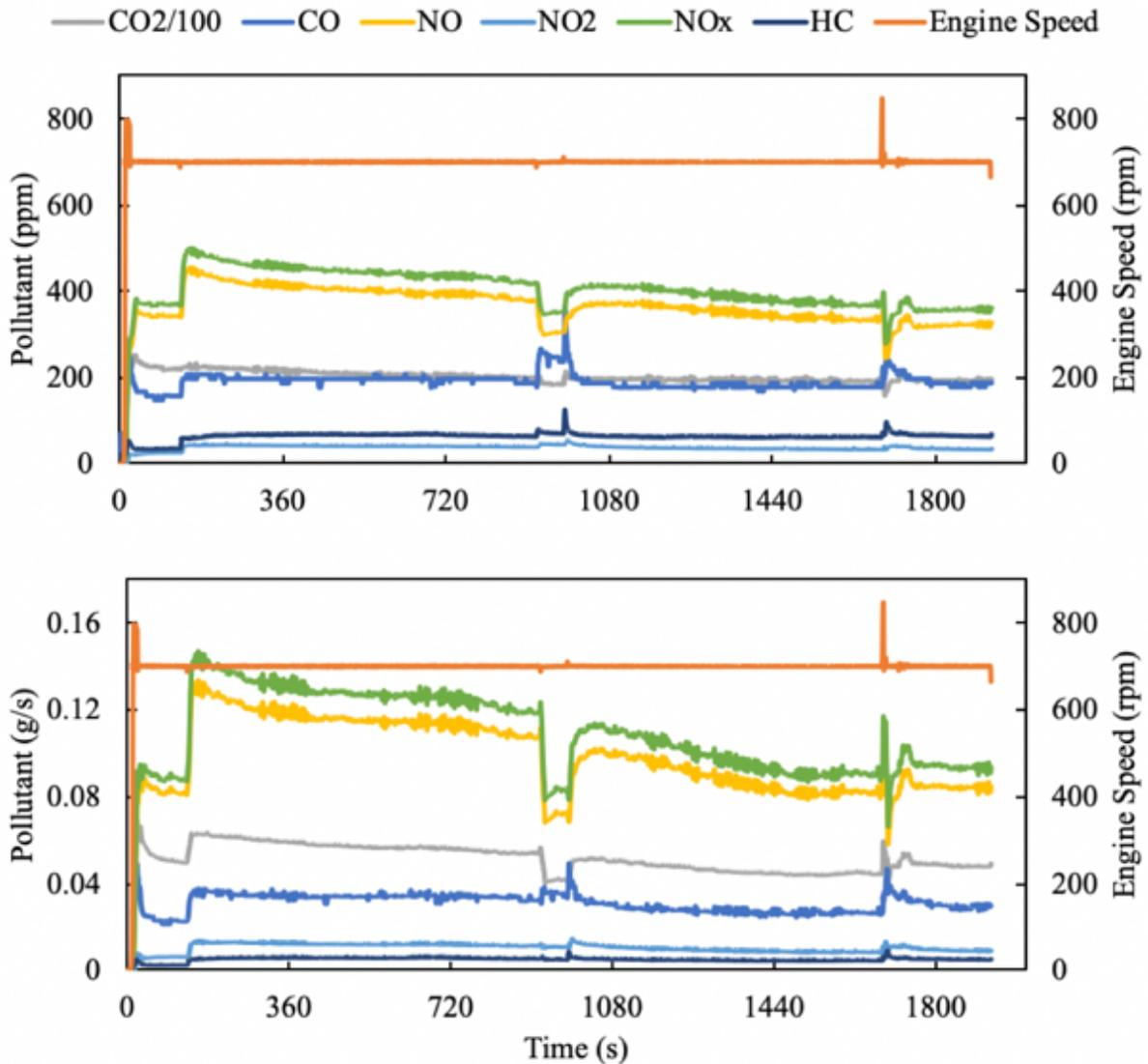
Gaseous emissions, in concentration and mass, and engine speed for the 1/23/19 cold start of Vessel A.
