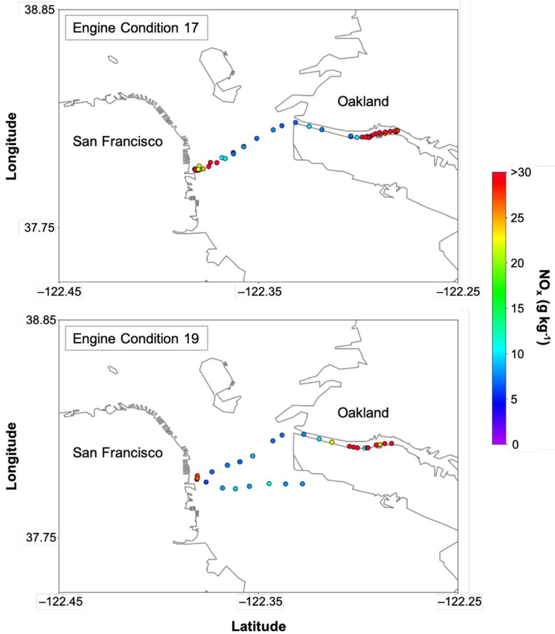
Map of NO<sub>x</sub> emission factors measured during engine conditions 17 and 19, in which the SCR was turned on but showed driving mode dependence for functionality. During the slow cruises in the Oakland Inner Harbor and maneuvering and docking at the three ferry docks, NO<sub>x</sub> emissions are elevated. During the steady cruises heading out of the harbor and across the SF Bay, emissions are lower.
