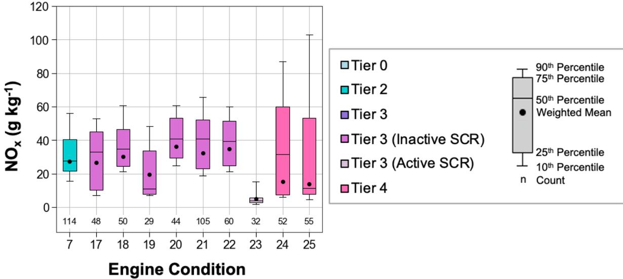
Note that NO<sub>x</sub> was not measured for all engine conditions, as summarized in Table 13. The noted sample size (n) refers to the number of emission factors included in each distribution.
