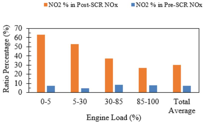
**Difference between Post- and Pre-SCR NO<sub>2</sub> divided by the Pre-SCR NO<sub>x</sub>.**
