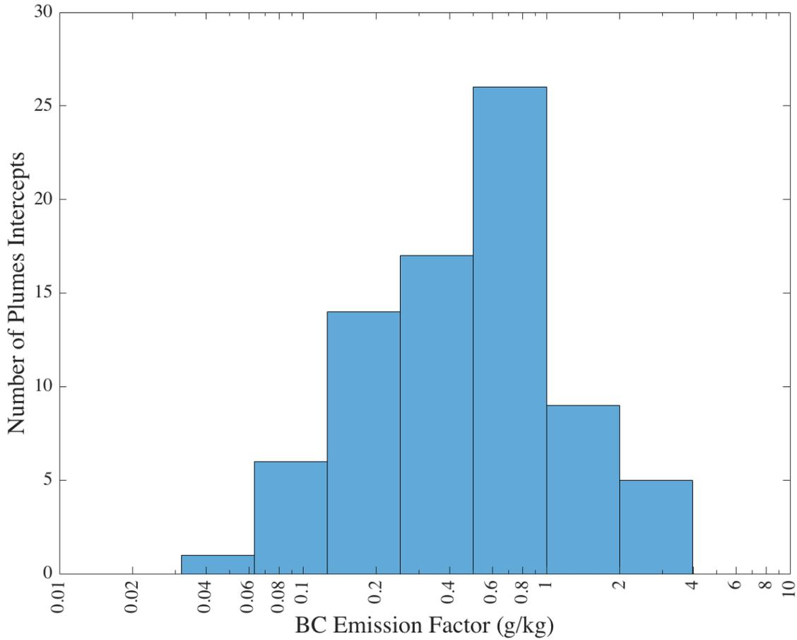
Distribution of BC emission factors from all onshore measurements. Note the log scale of the x-axis.
