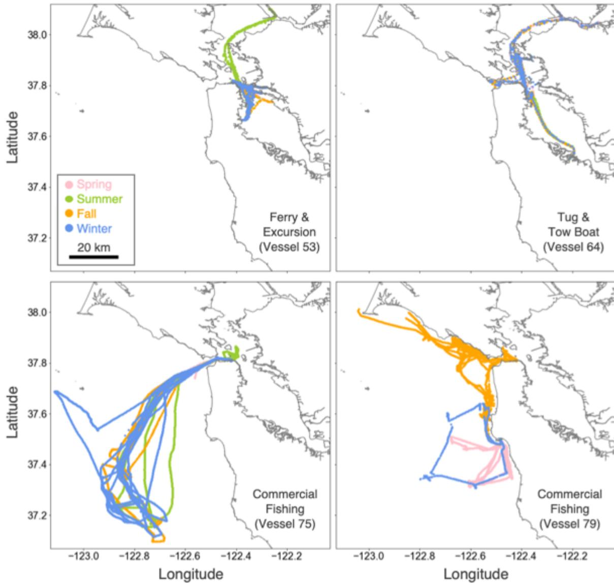
Examples of AIS-based vessel tracks for different vessel types operating in the San Francisco Bay Area. Each mapped point represents the vessel's reported AIS locational data in the specified ~30-day period for each season.
