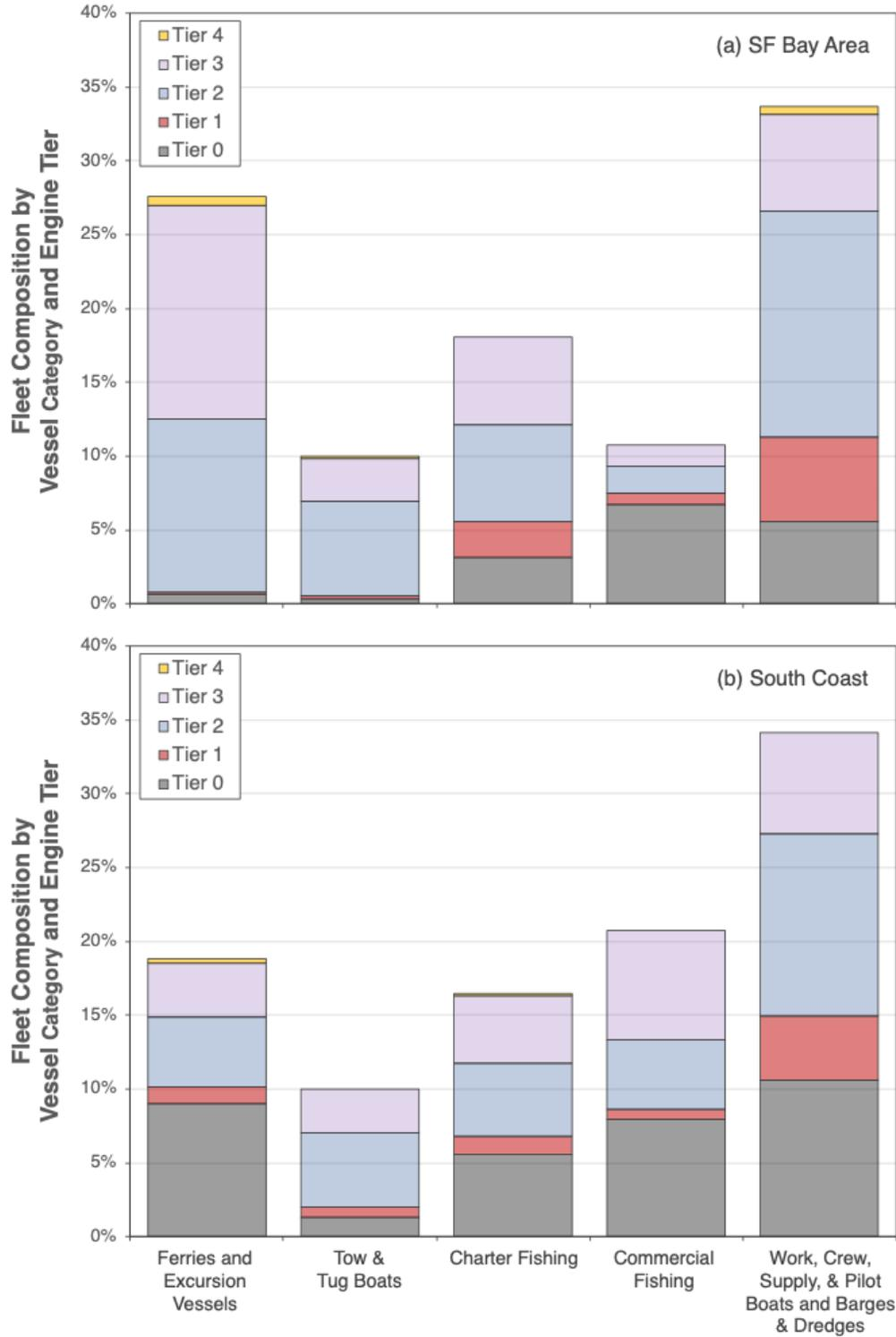
Composition of (a) SF Bay Area and (b) South Coast CHC fleets by engine tier, based on projected 2023 vessel count estimates (CARB, 2020). The fractional distributions are relative to the total fleet count in each area, such that the sum of all category bars equals 100%. Note that these plots are based on preliminary emission inventory data and are subject to change as updated information becomes available.
