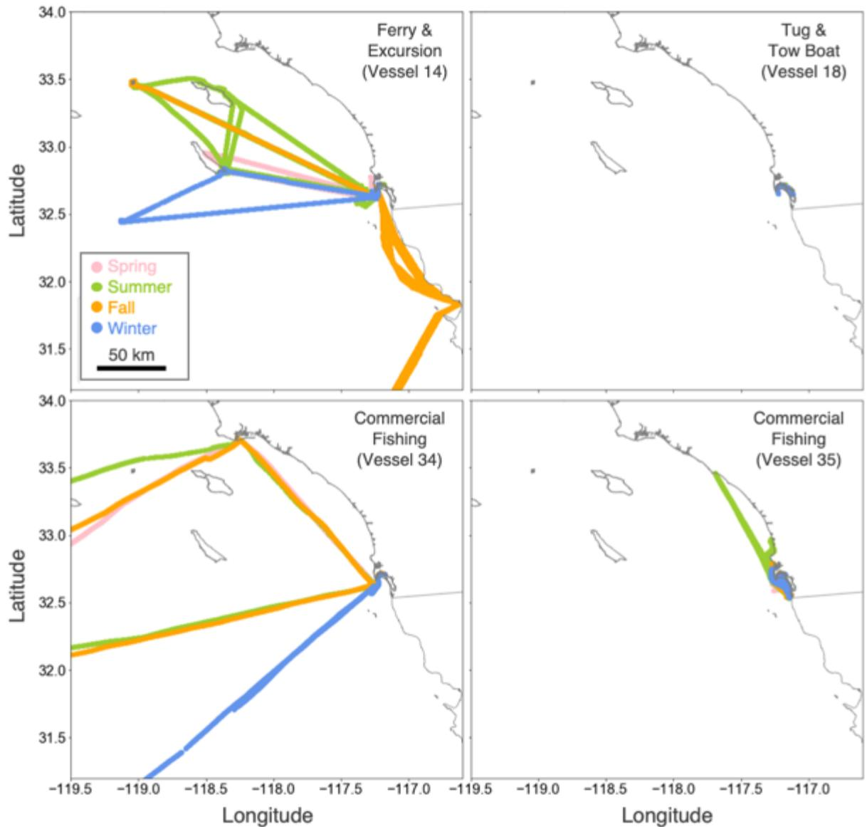
Examples of AIS-based vessel tracks for different vessel types operating in San Diego. Each mapped point represents the vessel's reported AIS locational data in the specified ~30-day period for each season.
