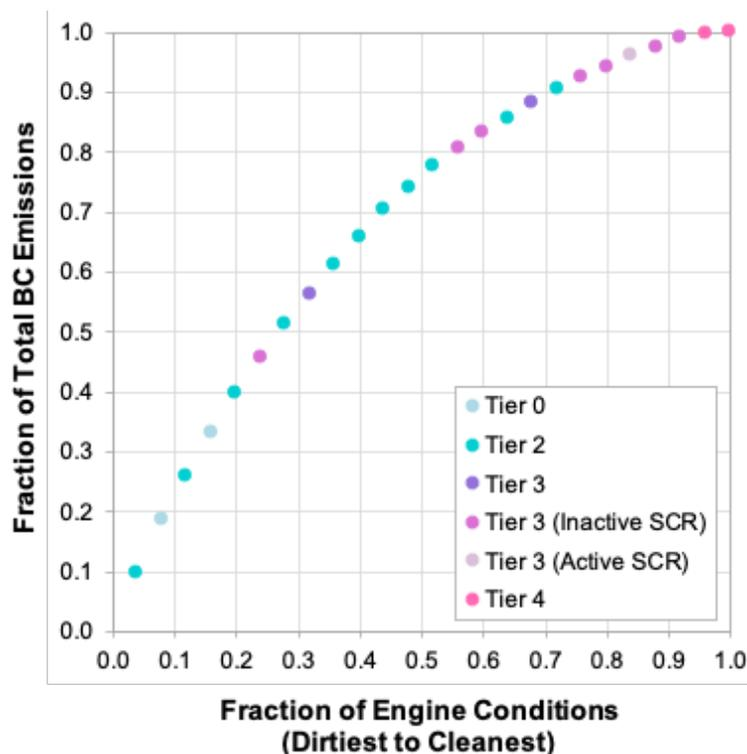
**Cumulative distribution of the overall BC emission factors for the 25 engine conditions included in this study. Emission factors are ranked from highest to lowest on the horizontal axis, and the corresponding cumulative BC emitted is shown on the vertical axis. Engine tier is noted for each measured engine condition. The overall BC emission factor was determined by a weighted average scheme described in the text above.**
