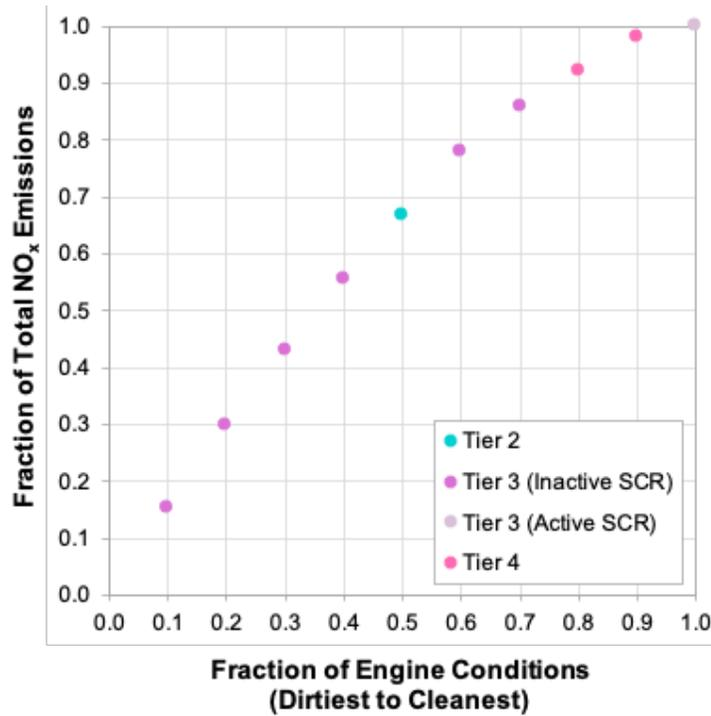
Cumulative distribution of overall NO<sub>x</sub> emission factors for the subset of 10 engine conditions with NO<sub>x</sub> measurements. The overall NO<sub>x</sub> emission factor was determined by a weighted average scheme described in the text above. Emission factors are ranked from highest to lowest on the horizontal axis, and the corresponding cumulative NO<sub>x</sub> emitted is shown on the vertical axis. Engine tier is noted for each measured engine condition.
