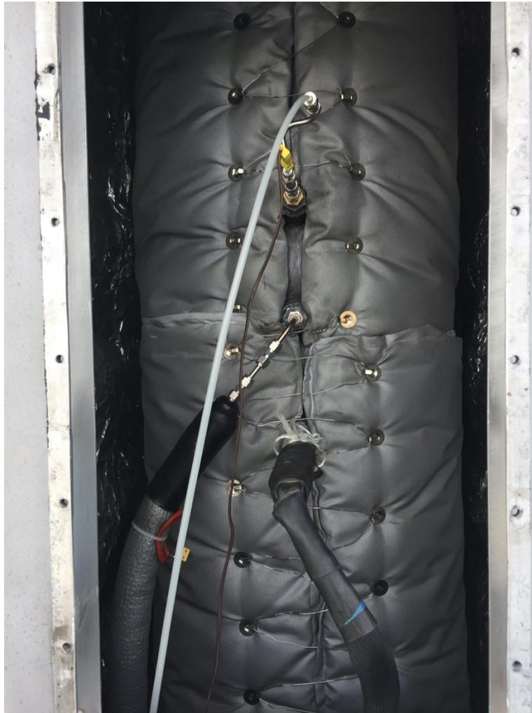
**Post-SCR sampling position on the second story deck of Vessel B.**
