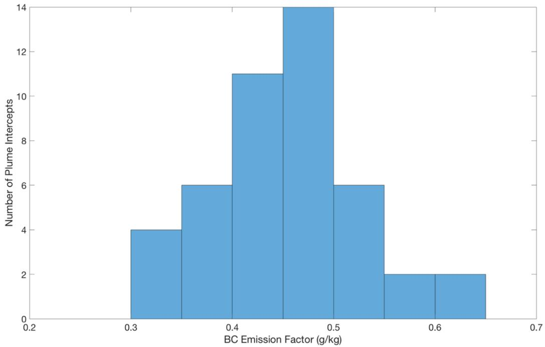
Distribution of BC emission factors (n = 58) measured on-board a Tier 2 passenger boat with wet exhaust.
