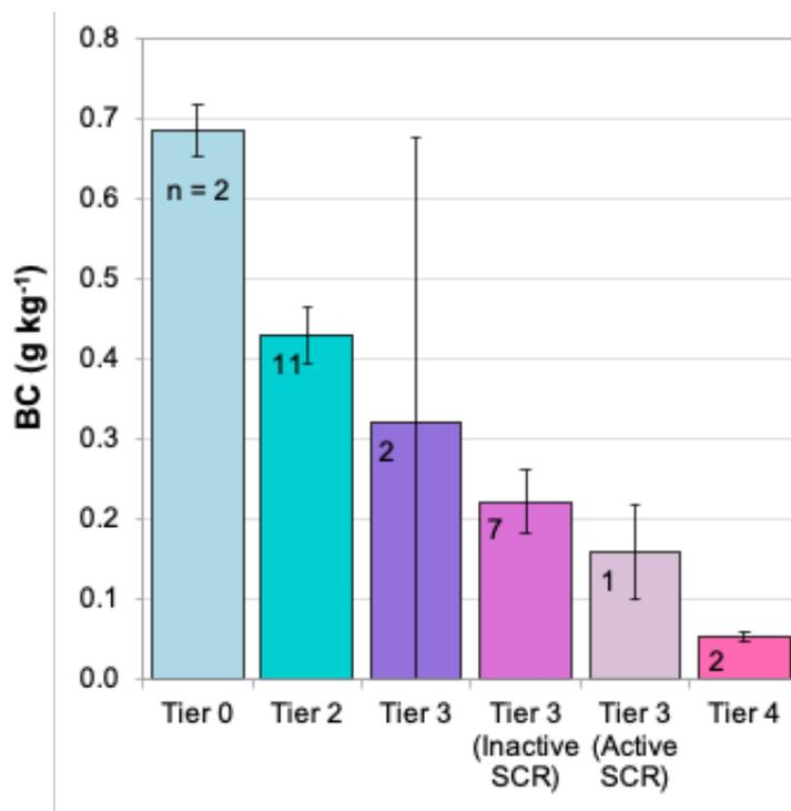
Overall BC emission factors ( $\pm$  95% confidence interval) by engine tier, as also summarized in Table 12. The number (n) of engine conditions included in each average value is noted in each bar. The overall BC emission factor was determined by a weighted average scheme described in the text above.
