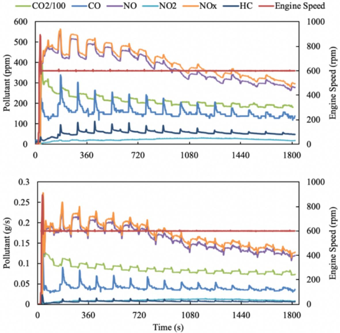
Vessel B gaseous emissions, in concentration and mass, for the 1/28/19 cold start. HC emissions were measured for each cold start but not during in-use operation.
