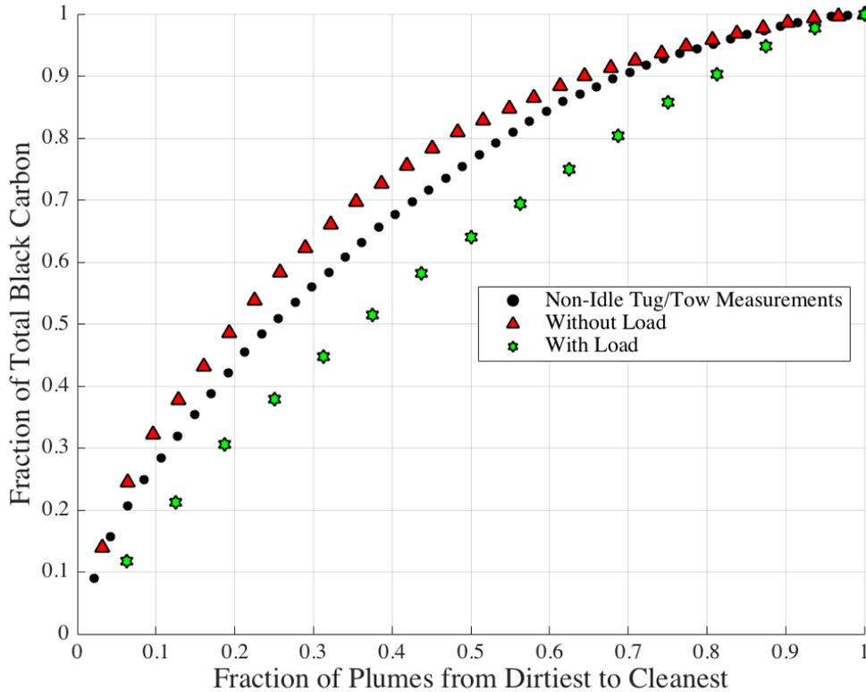
**Cumulative BC emission factor distributions of onshore measurements of tug and tow boats separated by operating mode.**
