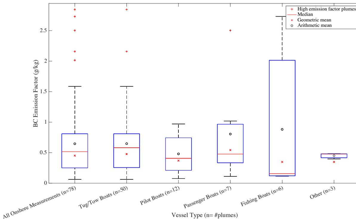
**Box plots of all onshore measurements separated by vessel type. High emission factor plumes are statistical outliers defined as emission factors greater than the 75<sup>th</sup> percentile of emission factors from that vessel type plus 1.5 times the interquartile range.**
