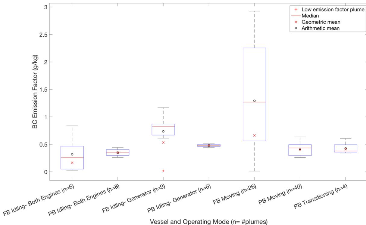
**Boxplots of emission factors from on-board measurements separated by vessel and operating mode. Fishing boat box plots are labeled FB and passenger boat box plots are labeled PB. Low emission factor plumes are statistical outliers. Outliers were identified when an emission factor was less than the 25<sup>th</sup> percentile of emission factors in that category minus 1.5 times the interquartile range.**
