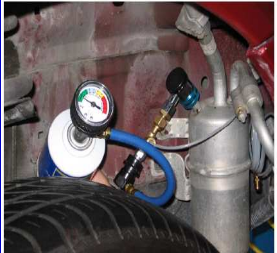
Figure 2: Small Can with Charge Kit and Adapter Installed on the Ford Focus Accumulator Service Port
