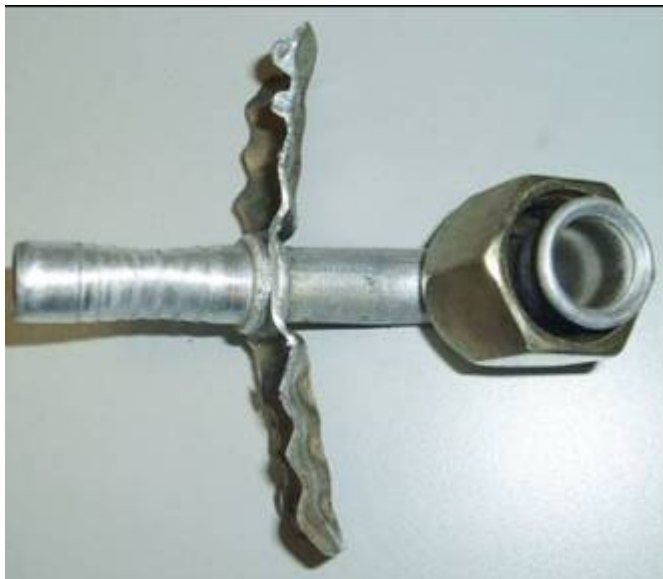
Necking down of crimp area due to incorrect crimp and incorrect fitting/hose selection
