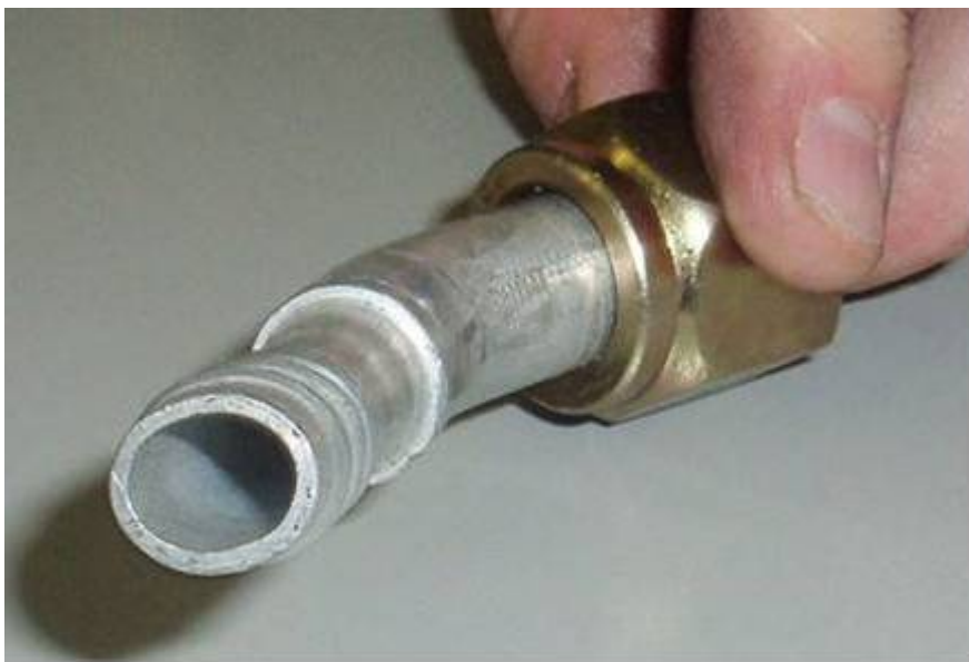
Incorrect tube and hose combination causing tube to seriously deform
