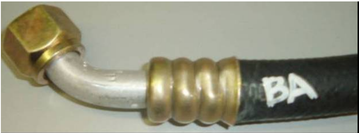
Tube and hoses blade finger style; crimp not overlapping
