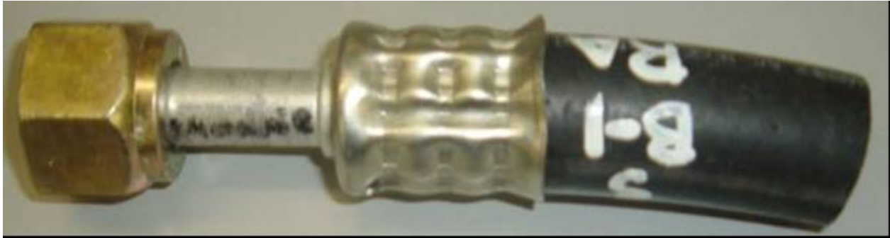
Incorrect 6 jaw method (crimped, rotated, re-crimped)
