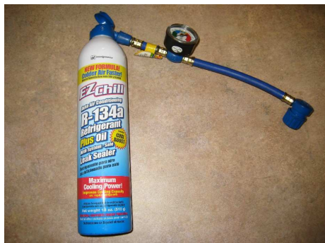
Can equipped with a valve and pressure gauge
