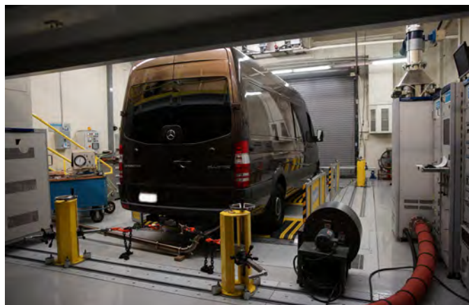
A Daimler Sprinter van tested on a dynamometer in CARB's laboratory.
