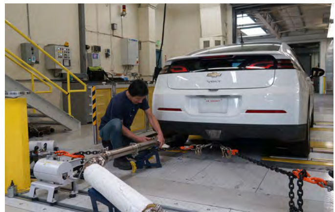
A Chevy Volt being set up for testing on a chassis dynamometer.
