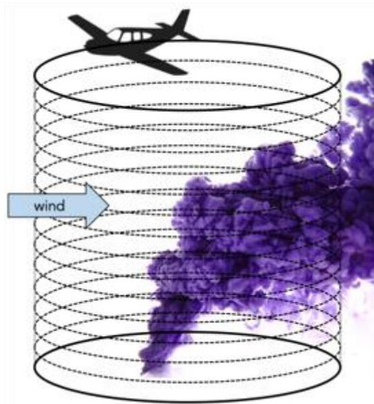
Figure 1. Theoretical flight path around a plume emitted from the surface. The cylindrical flight path and wind direction are shown.
