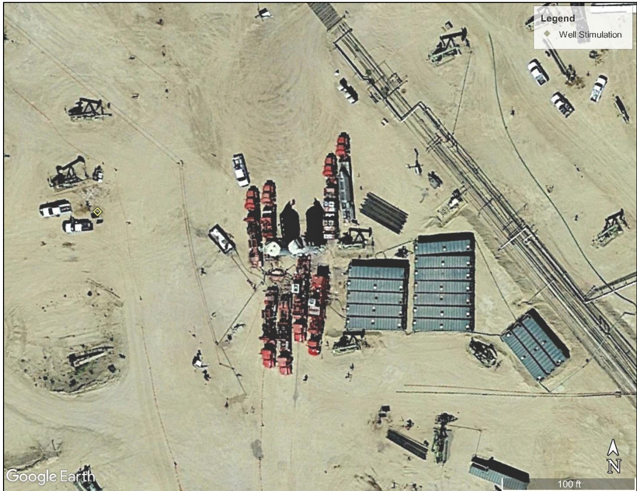
Figure 2. Hydraulic fracturing and other well stimulation treatments (WST) require the use of trucks, pumps, and other equipment that can produce air emissions. Shown is one of the hydraulic fracturing treatment in the Central Valley of California photographed by Google Earth. Red mixing and pump trucks can be seen next to rectangular and circular water, sand, and chemical storage and blending tanks. Pump-jacks, located at adjacent wells, and white pickup trucks are ubiquitous features on oil fields in California.
