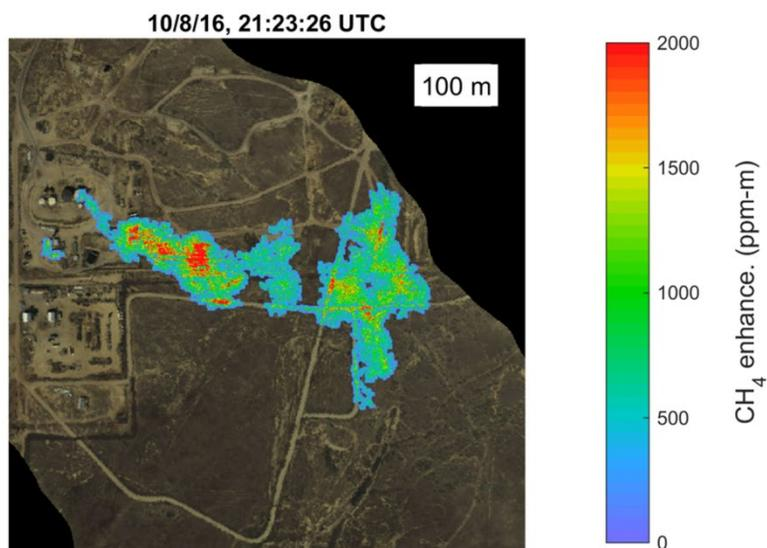
Figure 29: Airborne methane source mapping example in CA
