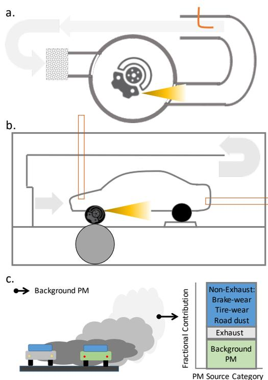
Figure 26: Diagram comparing various methods for characterizing brake-wear emissions: a) enclosed brake-dynamometer, b) sealed RL-SHED, leveraging full vehicle chassis dynamometers, and c) roadside studies.
