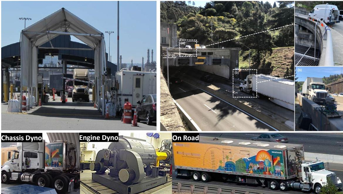
Figure 20: Pictures of various measurement platforms utilized to measure heavy-duty vehicle emissions
