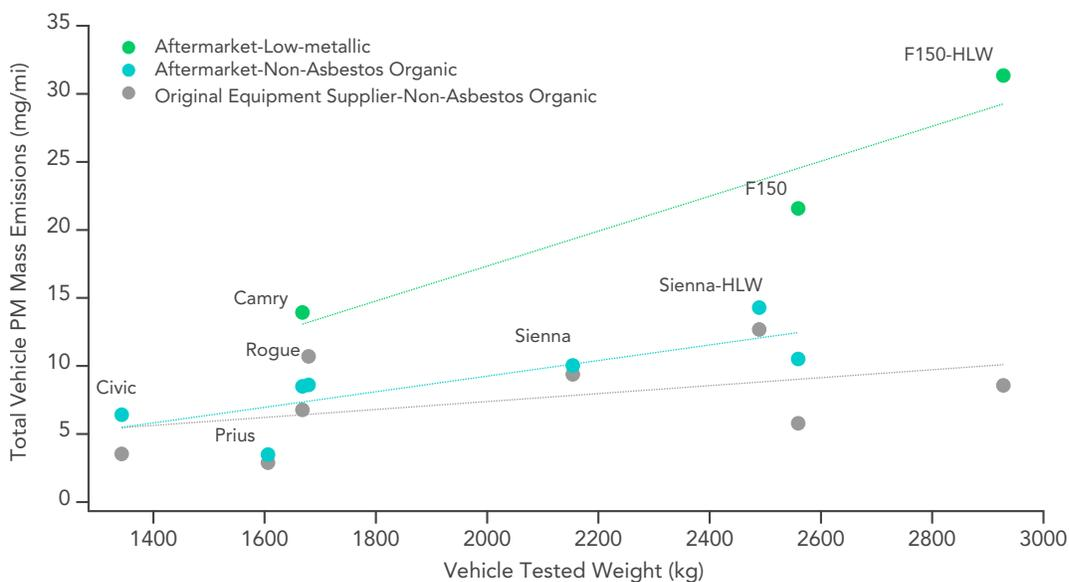
Figure 27: Total vehicle PM mass emissions for all vehicle tests and as a function of vehicle weight and brake pad material.
