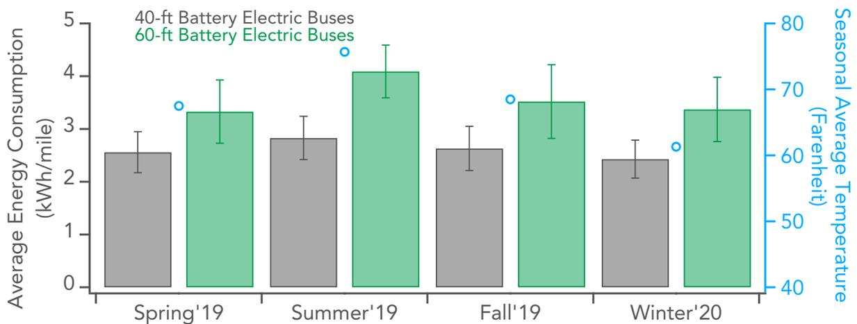
Figure 24: Energy consumption of battery electric buses operated in Lancaster, CA over different seasons
