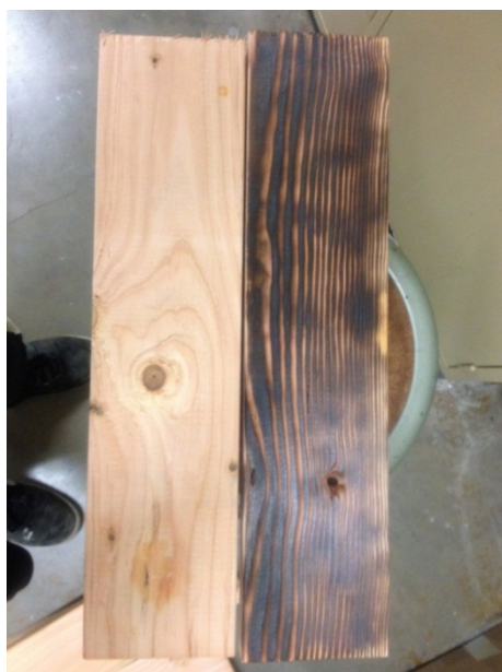
Figure 1: Photograph of a wood panel before (left) and after (right) being subjected to the flame from Coleman burner
