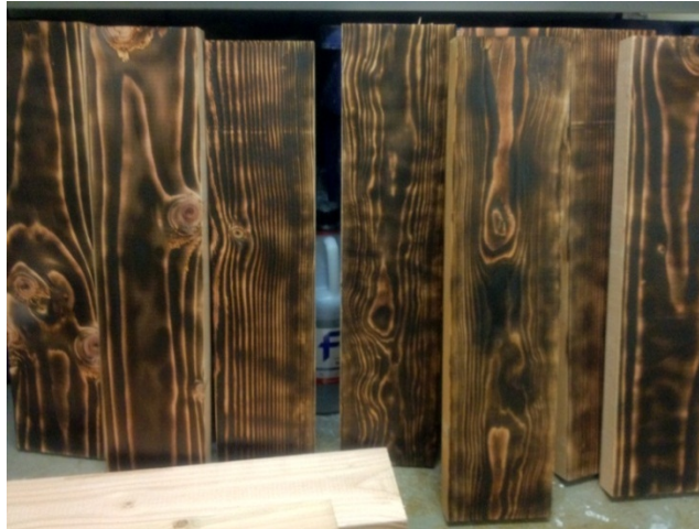
Figure 2: Photograph of a batch of wood panels after being subjected to the flame from Coleman burner
