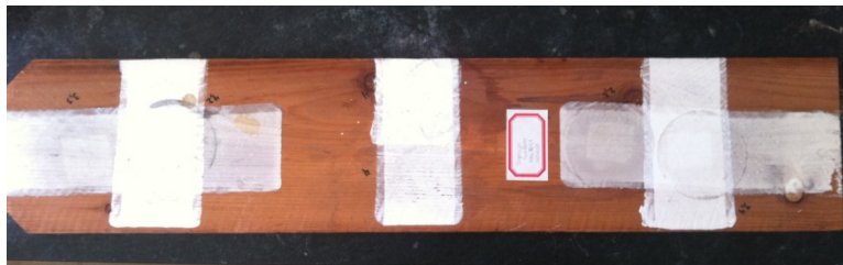
Figure 5. Photograph of a redwood panel (12"x36") prepared for tannin blocking test
