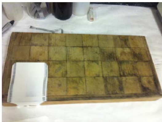
Figure 4. Photograph of a water damaged wood panel recovered from a residence in San Luis Obispo, CA. One of the test primers has been applied on the panel.
