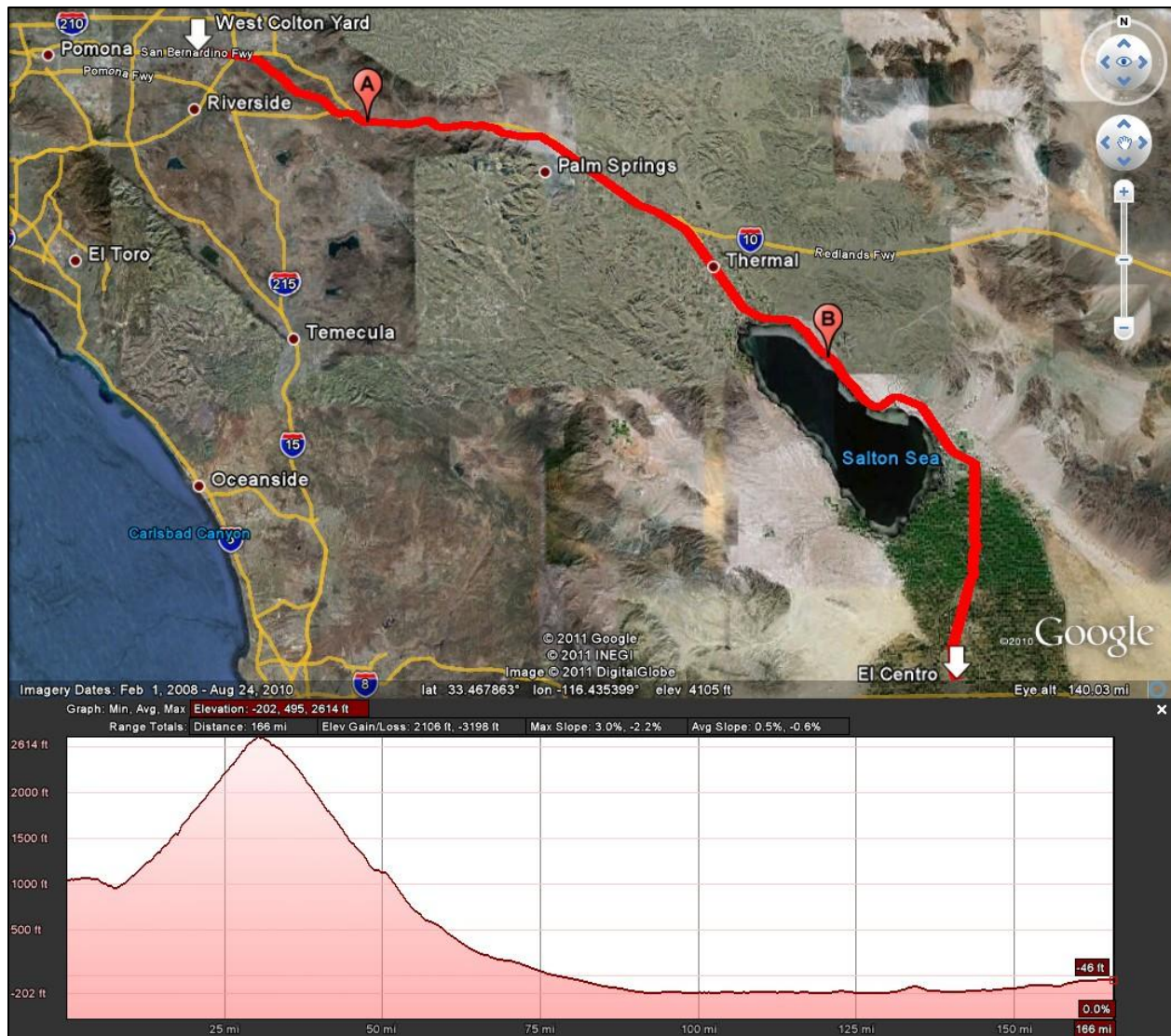
FIGURE 18. PATHWAY AND ELEVATION PROFILE OF WEST COLTON - EL CENTRO SERVICE ROUTE
