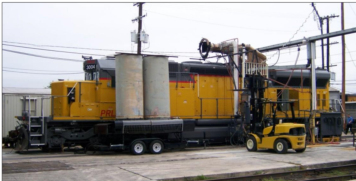
FIGURE 7. TEST SETUP FOR PRLX3004 WITH AFTERTREATMENT
