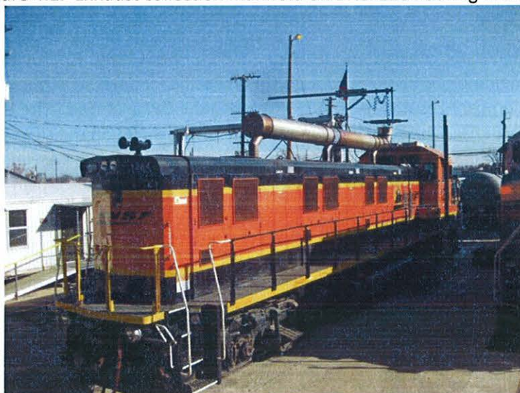
Figure 4.1: Exhaust collection manifold on BNSF1284 during final test
