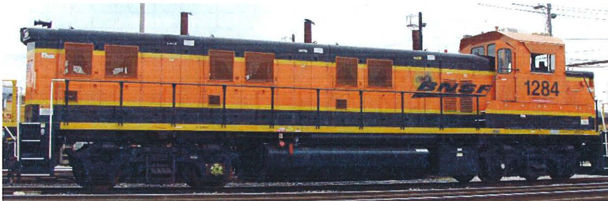
Figure 5. BNSF1284 With GT Exhaust DPF's Installed
