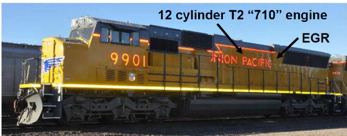
Figure 3. Re-powered SD59MX locomotive with EGR in 2011.
