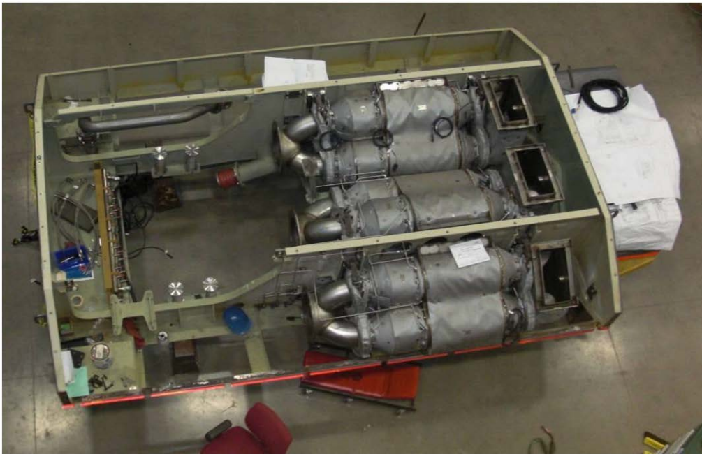
Figure 6. EMD Aftertreatment Tray build up prior to application on locomotive
