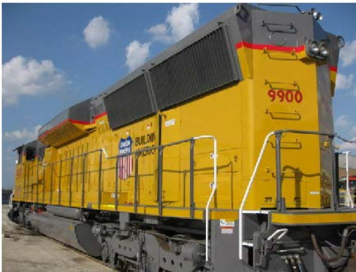
Figure 8. Overhang of DOC/DPF “tray” on engine compartment at mid-locomotive (Electro-Motive Diesel, Inc., Copyright ©, March 01, 2012).
