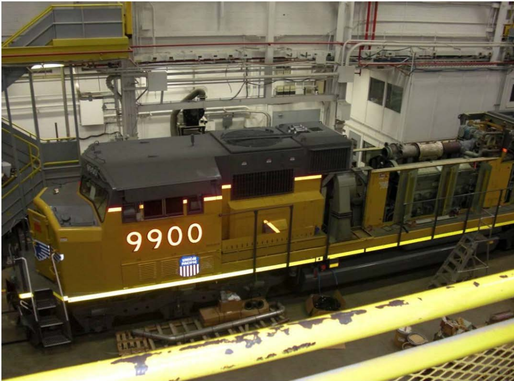
Figure 4. EMD 9900 with engine hood removed.
