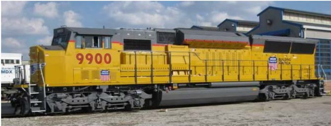
Figure 7. SD59MX UP 9900 with EGR and DOC/DPF “tray” (Electro-Motive Diesel, Inc., Copyright ©, March 01, 2012).
