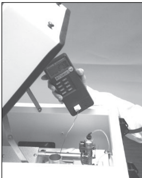
Figure AS.11 Filter Temperature Check in a Model 2025 or 2025i
