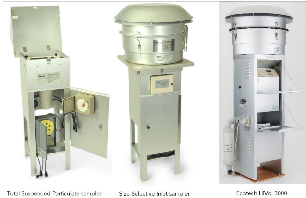
Figure AS.1 Examples of TSP and SSI Samplers
