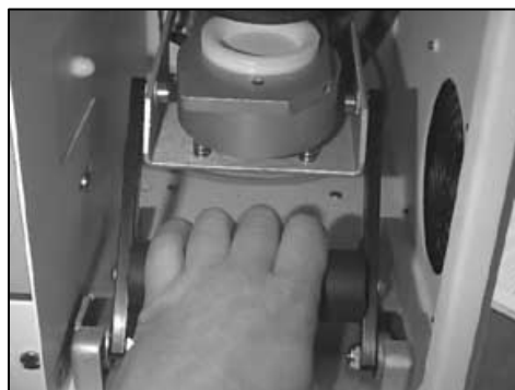
Figure AS.8 Lowering the Filter Platform of a Partisol 2000/2000i
