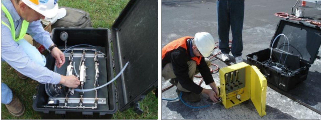
Figure 29 – View of the LFE and flow meters devices
