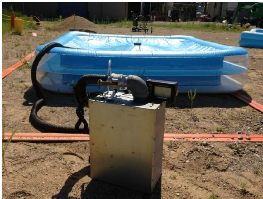
Figure 3 – Capturing gas leak area for rate measurements
