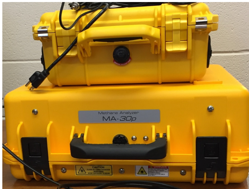
Figure 5 – LGR-UGGA Methane Analyzer and Battery Pack
