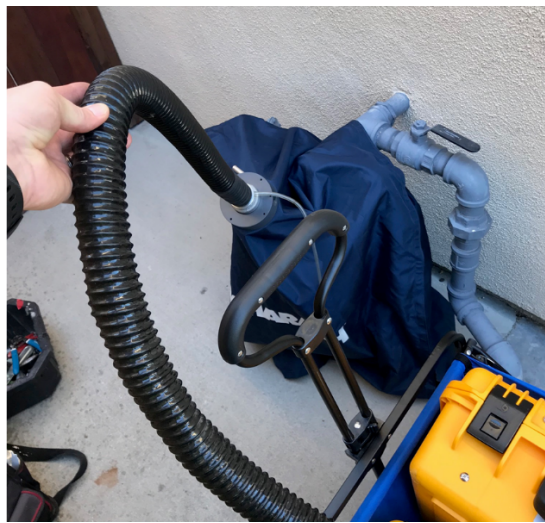
Figure 8 – Example of meter measurements with the Hi-Flow device and LGR-UGGA
