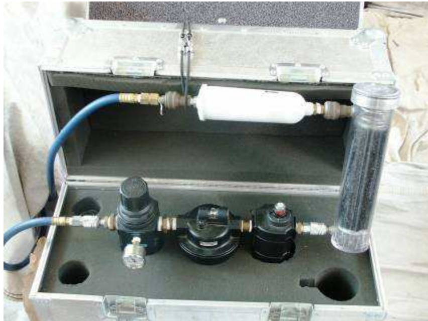
Figure 8-2 Field Processing Unit for Purifying Dilution Air in Carrying Case
