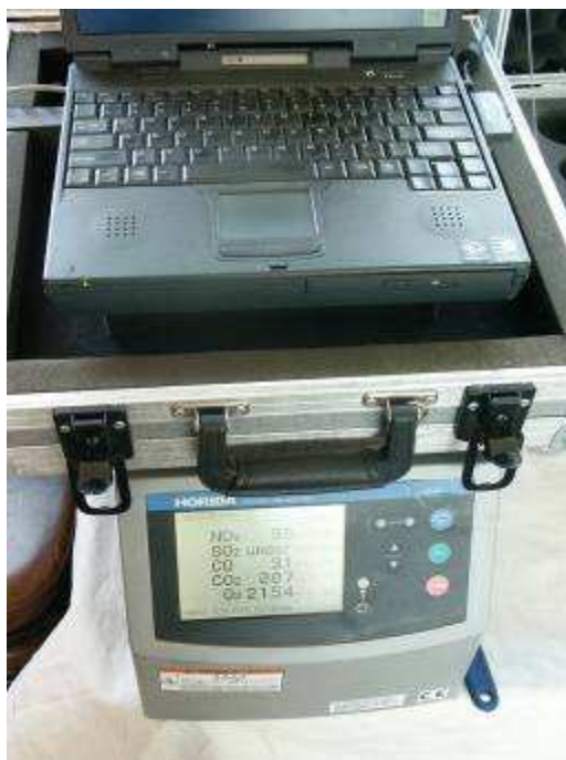
Figure 8-3 In-Field Illustration of Continuous Gas Analyzer and Computer for Data Logging
