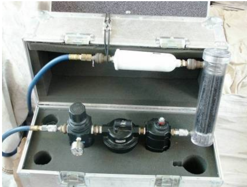
Figure 2: Field Processing Unit for Purifying Dilution Air in Carrying Case
