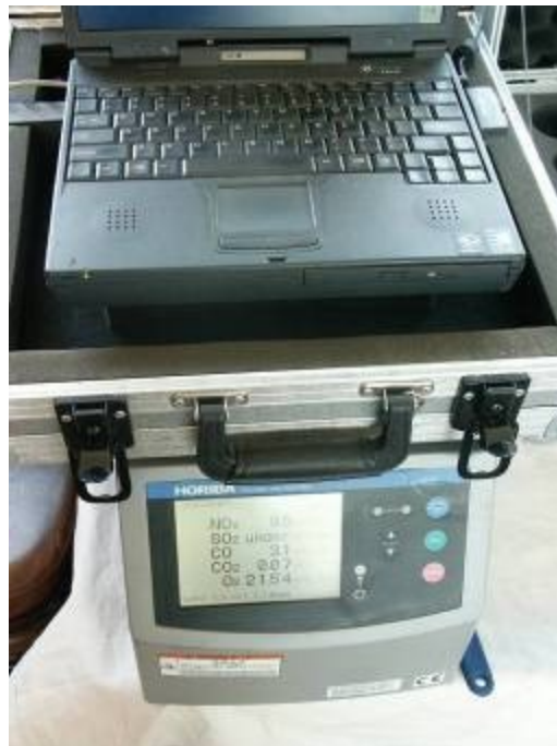
Figure 3: In-field Illustration of Continuous Gas Analyzer and Computer for Data Logging
